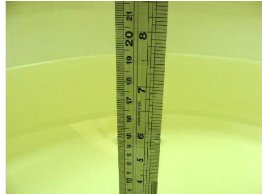
Fig 7.2 Photo of Liquid Height for Body SAR
