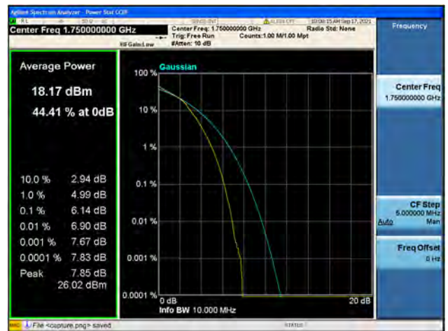
Band4 / 10MHz / High CH / 64QAM
