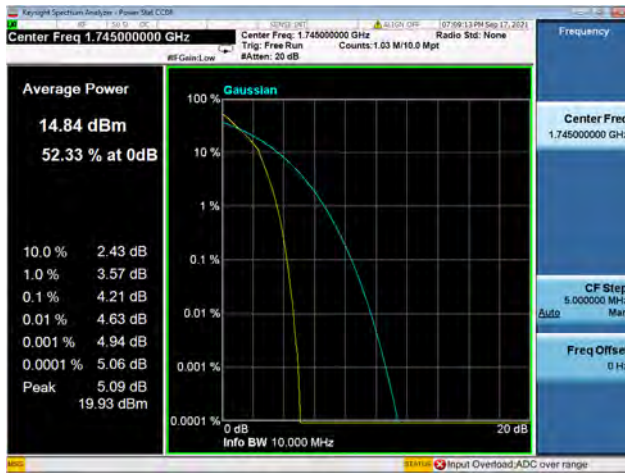
Band66 / 10MHz / Mid CH / 64QAM
