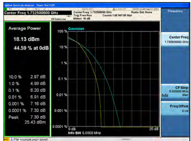
Band4 / 1.4MHz / Mid CH / 64QAM
