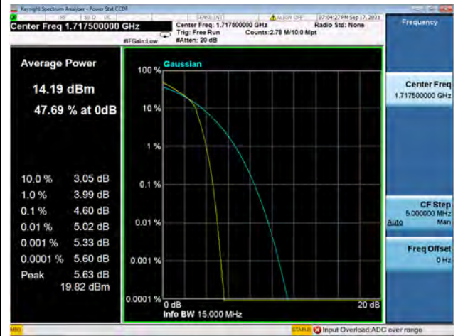
Band66 / 15MHz / Mid CH / QPSK
