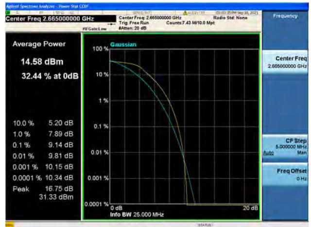
Band41 / 20MHz / High CH / 64QAM
