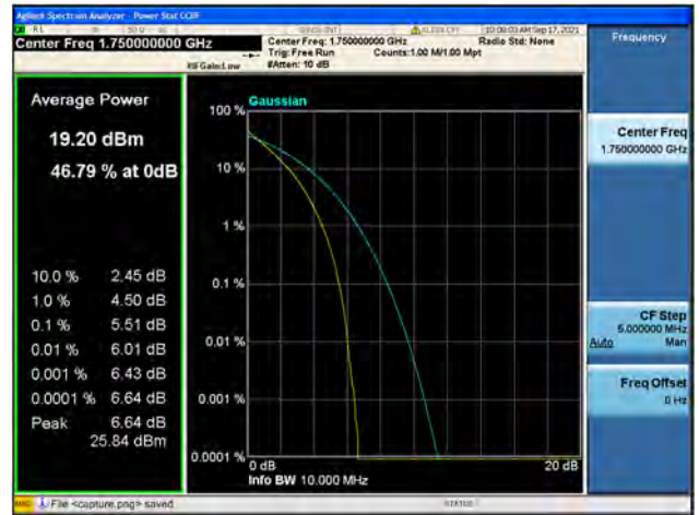
Band4 / 10MHz / High CH / 64QAM
