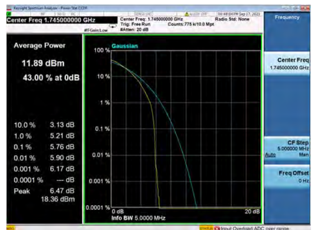
Band66 / 1.4MHz / Mid CH / 64QAM
