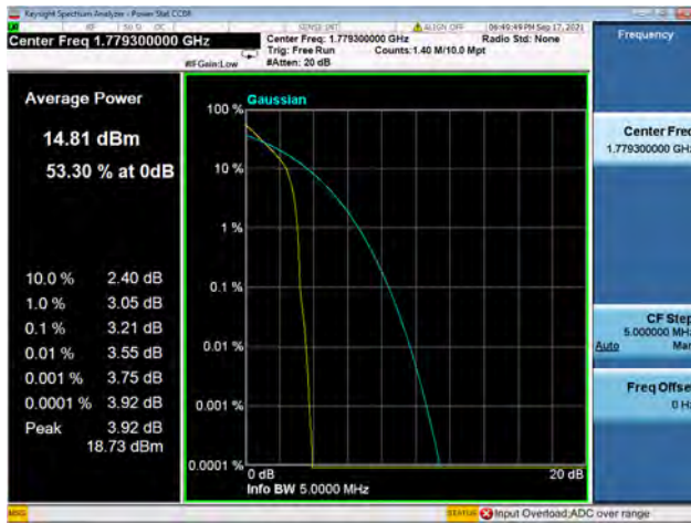
Band66 / 1.4MHz / High CH / 64QAM
