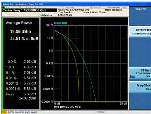
Band4 / 3MHz / High CH / 16QAM
