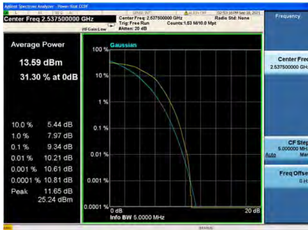
Band41 / 5MHz / Mid CH / 16QAM
