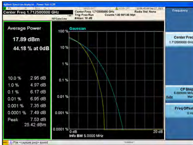
Band4 / 5MHz / Mid CH / 16QAM
