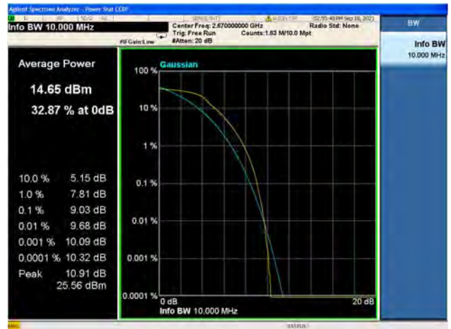
Band41 / 10MHz / High CH / 64QAM
