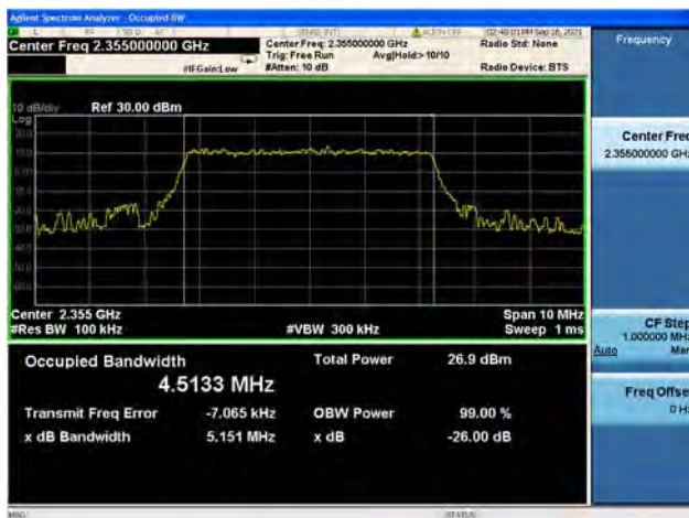
Band40/ Block B / 5MHz / Mid CH / 16QAM
