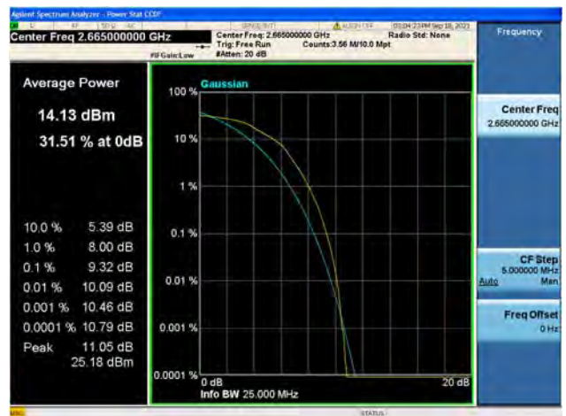
Band41 / 20MHz / High CH / 64QAM
