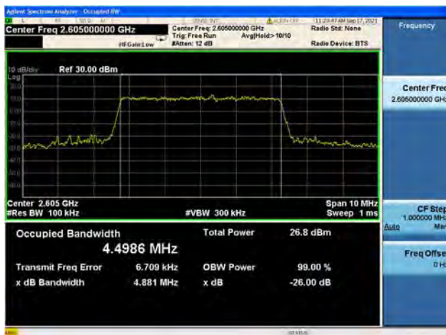
Band41 / 5MHz / Mid CH / 16QAM
