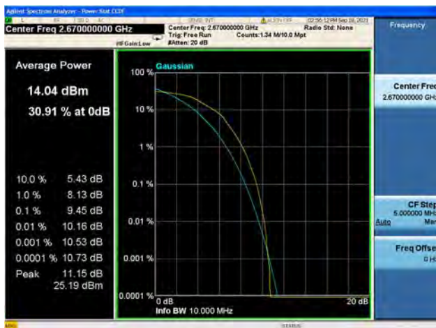
Band41 / 10MHz / High CH / 16QAM
