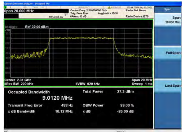
Band40/ Block A / 10MHz / Mid CH / 64QAM
