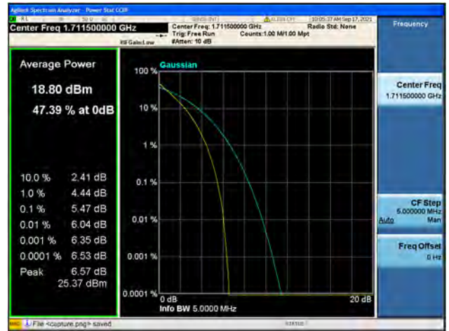
Band4 / 3MHz / Low CH / 64QAM
