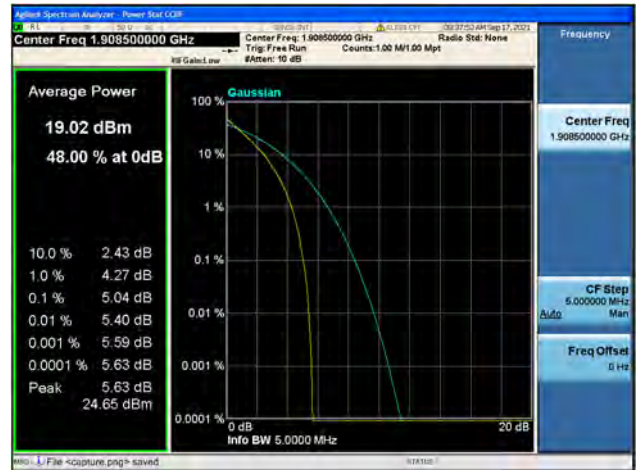
Band2 / 3MHz / High CH / 64QAM
