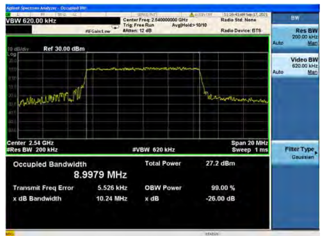
Band41 / 10MHz / Low CH / 64QAM
