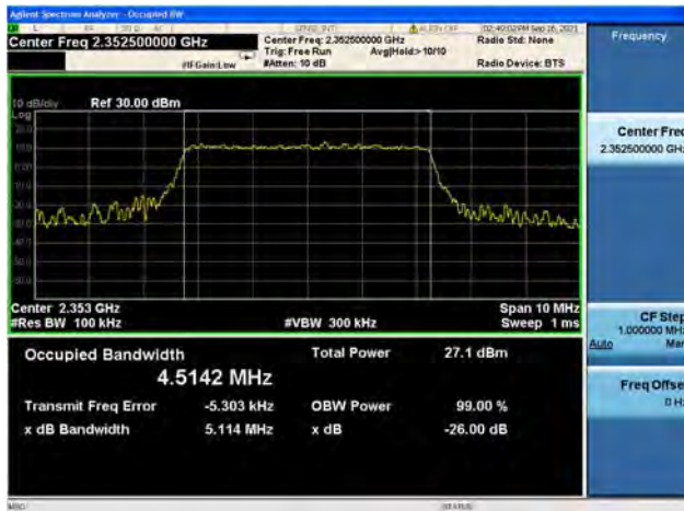
Band40/ Block B / 5MHz / Mid CH / 16QAM
