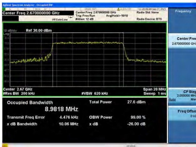
Band41 / 10MHz / High CH / 16QAM
