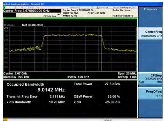
Band41 / 10MHz / High CH / 64QAM
