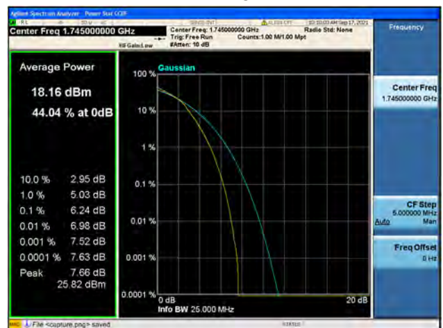
Band4 / 20MHz / High CH / 64QAM
