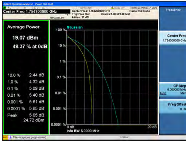
Band4 / 1.4MHz / High CH / 64QAM
