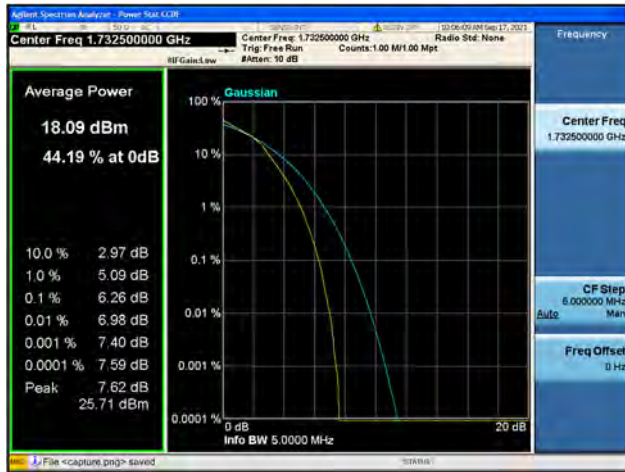
Band4 / 3MHz / High CH / 16QAM
