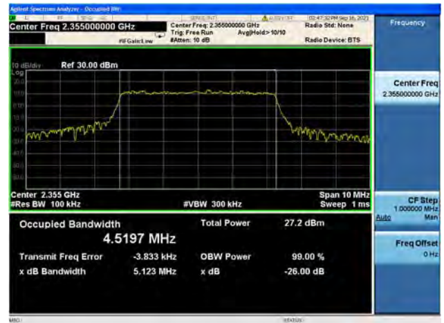
Band40/ Block B / 5MHz / Mid CH / 64QAM
