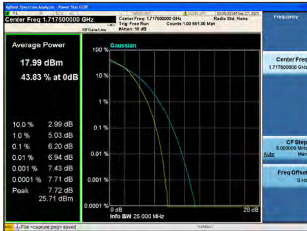
Band4 / 15MHz / Mid CH / 16QAM
