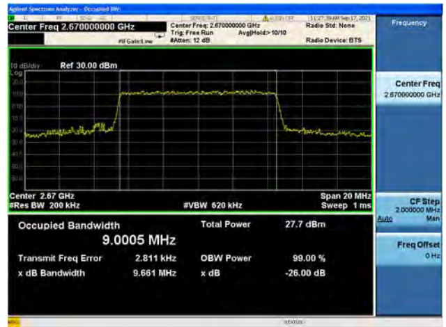
Band41 / 10MHz / High CH / 64QAM
