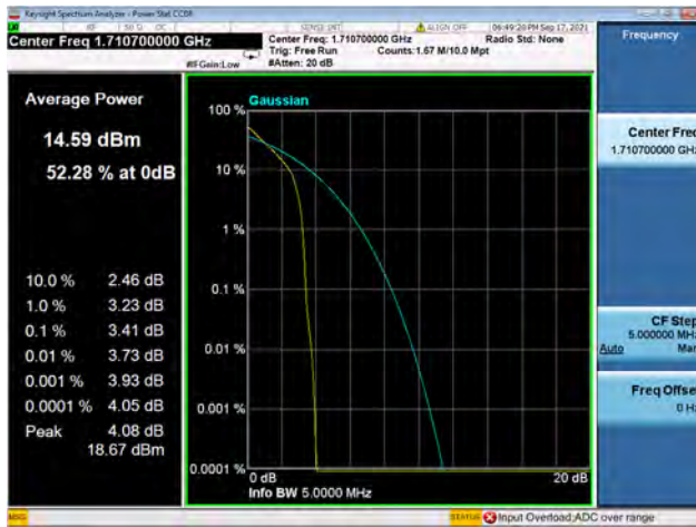
Band66 / 1.4MHz / Low CH / 64QAM
