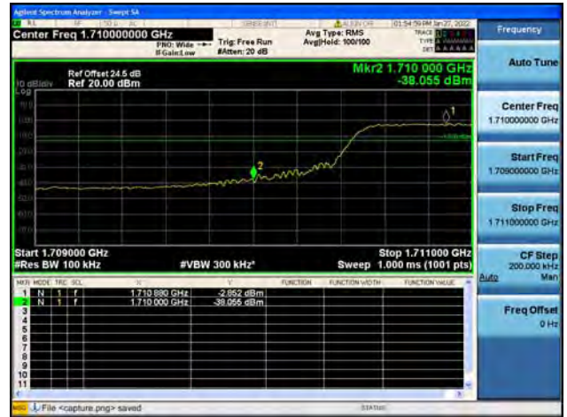
Band66 / 10MHz / High CH / QPSK / FULL RB
