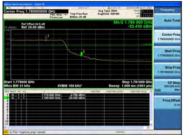
Band66 / 5MHz / High CH / QPSK / FULL RB
