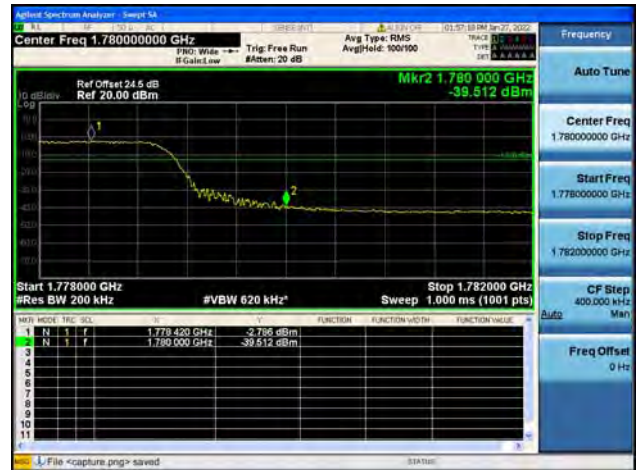
Band66 / 20MHz / High CH / QPSK / FULL RB
