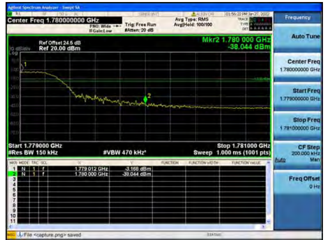
Band66 / 15MHz / High CH / QPSK / FULL RB
