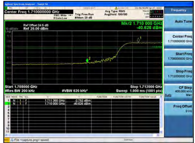
Band66 / 20MHz / High CH / QPSK / FULL RB
