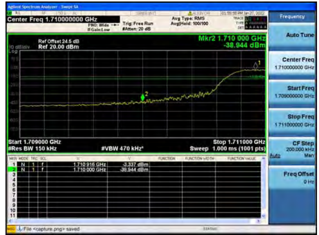
Band66 / 15MHz / High CH / QPSK / FULL RB
