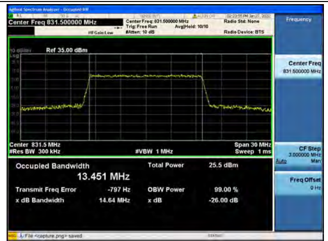
Band26Part22 / 15MHz / Mid CH / 16QAM
