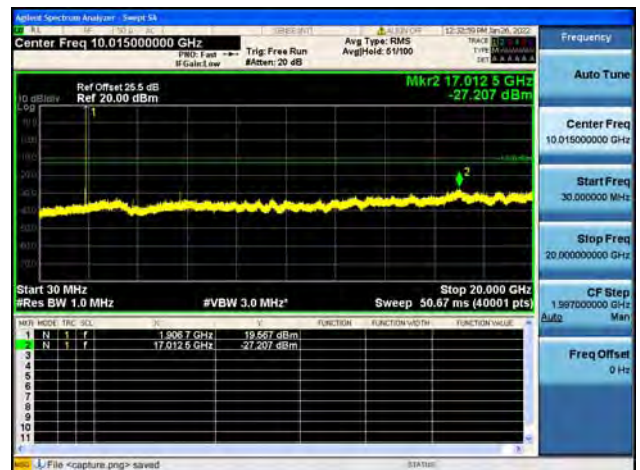
Band2 / 3MHz / High CH / 16QAM
