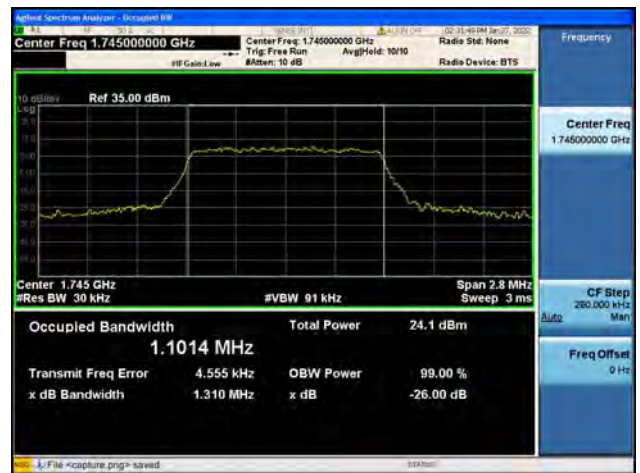
Band66 / 1.4MHz / High CH / 16QAM
