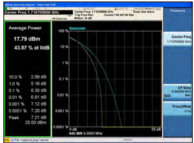
Band66 / 1.4MHz / Mid CH / 16QAM
