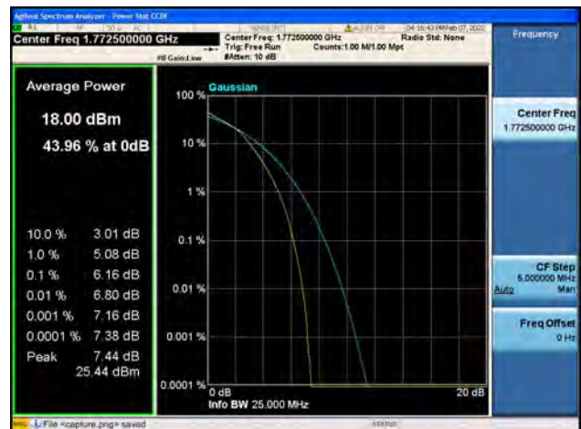
Band66 / 15MHz / High CH / 16QAM
