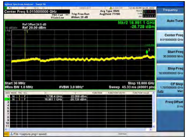
Band4 / 5MHz / High CH / 16QAM
