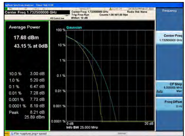
Band4 / 20MHz / High CH / 16QAM
