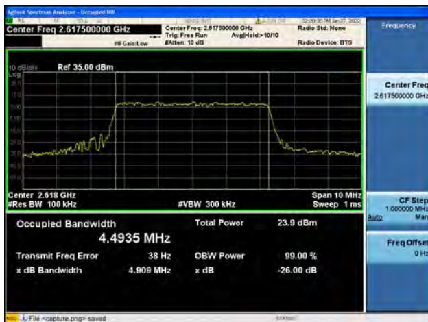
Band38 / 5MHz / High CH / QPSK
