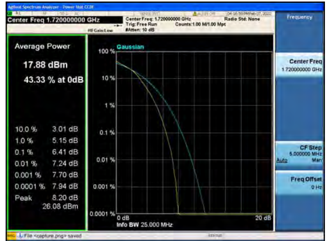
Band66 / 20MHz / Mid CH / 16QAM
