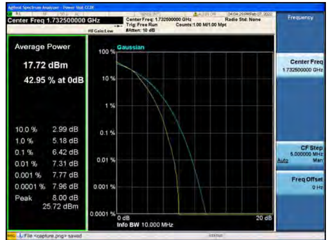
Band4 / 10MHz / High CH / 16QAM
