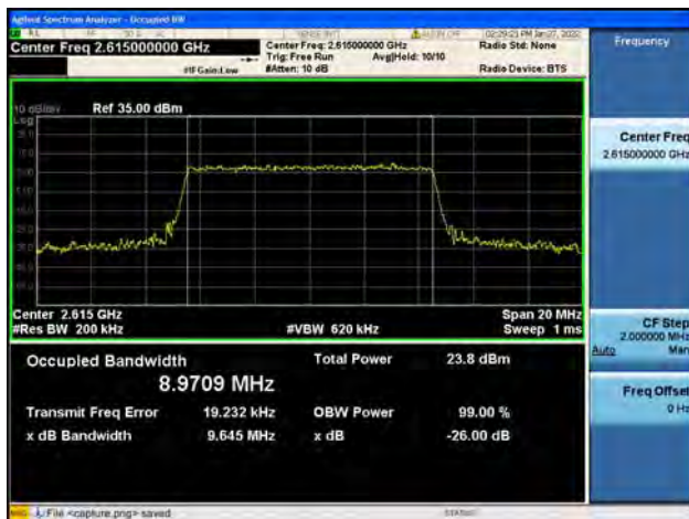
Band38 / 10MHz / High CH / QPSK
