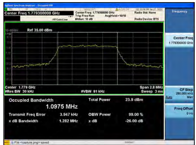
Band66 / 1.4MHz / High CH / 16QAM
