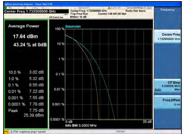
Band4 / 3MHz / High CH / 16QAM
