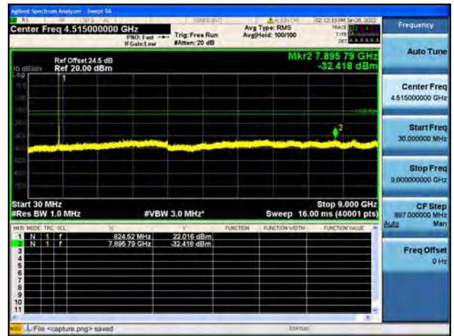
Band5 / 3MHz / Mid CH / 16QAM
