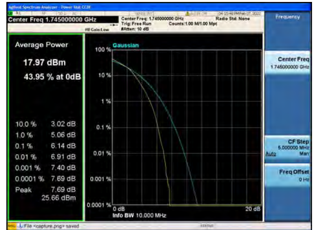
Band66 / 10MHz / High CH / 16QAM
