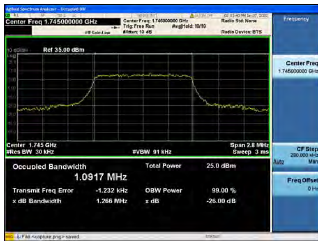
Band66 / 1.4MHz / High CH / QPSK
