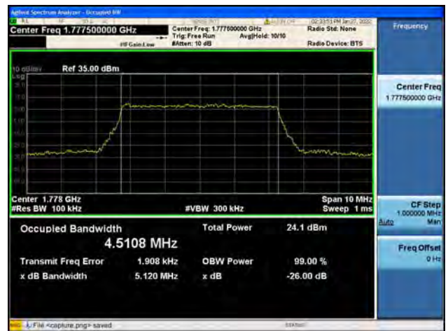
Band66 / 5MHz / High CH / 16QAM
