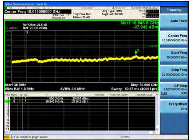
Band2 / 3MHz / Mid CH / 16QAM
