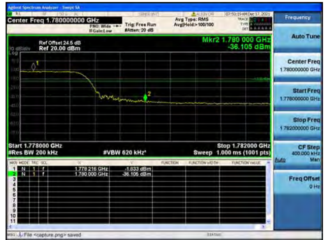
Band66 / 20MHz / High CH / QPSK / FULL RB
