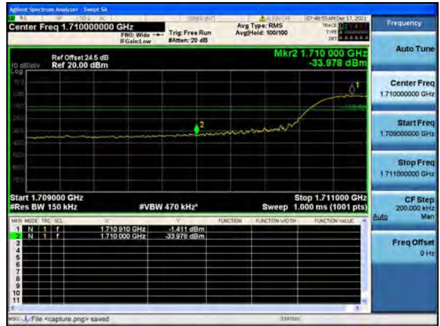
Band66 / 15MHz / High CH / QPSK / FULL RB
