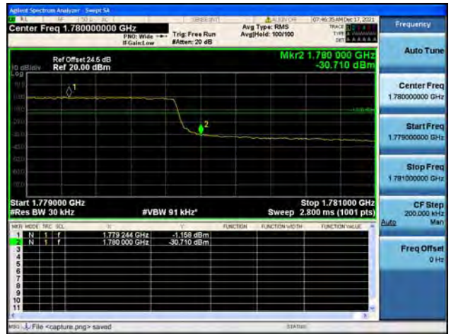
Band66 / 3MHz / High CH / QPSK / FULL RB
