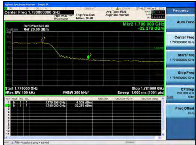
Band66 / 10MHz / High CH / QPSK / FULL RB
