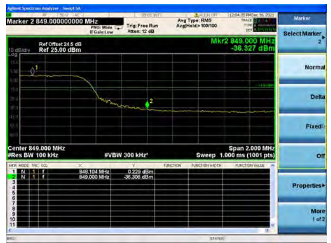
Band26 / 10MHz / High CH / QPSK / FULL RB
