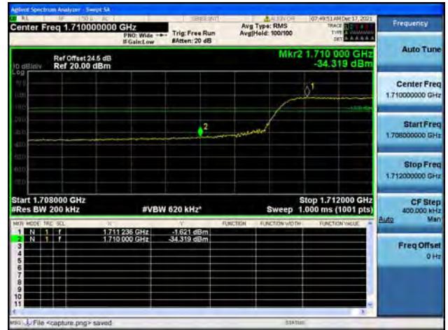
Band66 / 20MHz / High CH / QPSK / FULL RB
