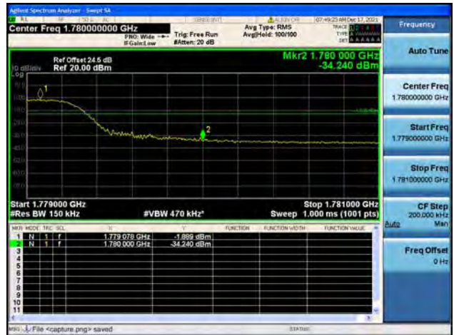
Band66 / 15MHz / High CH / QPSK / FULL RB
