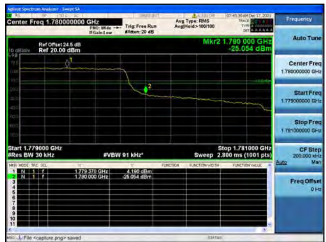
Band66 / 1.4MHz / High CH / QPSK / FULL RB
