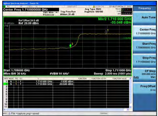
Band66 / 3MHz / High CH / QPSK / FULL RB
