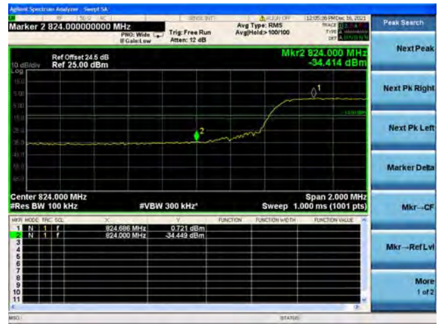
Band26 / 10MHz / High CH / QPSK / FULL RB
