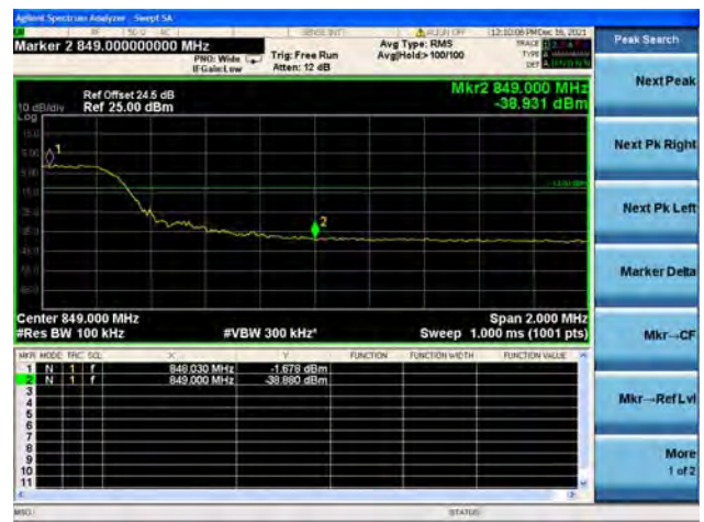
Band26 / 15MHz / High CH / QPSK / FULL RB
