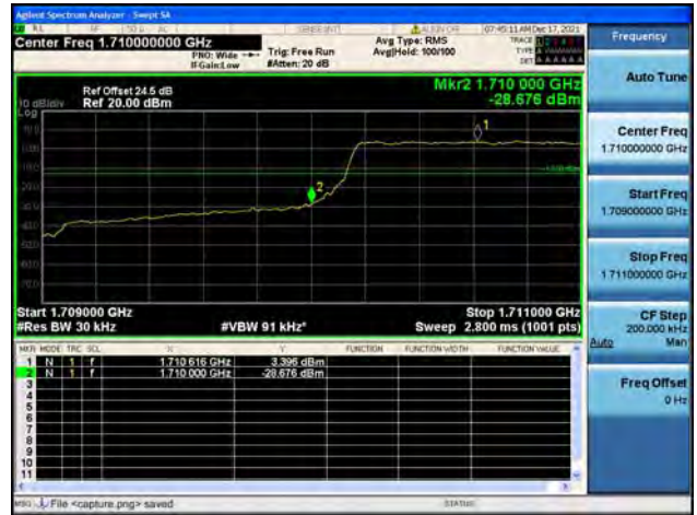
Band66 / 1.4MHz / High CH / QPSK / FULL RB
