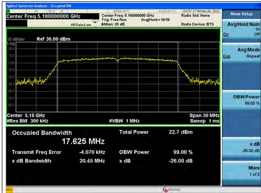
(Channel 36, 5180MHz, 802.11ac (VHT20))
