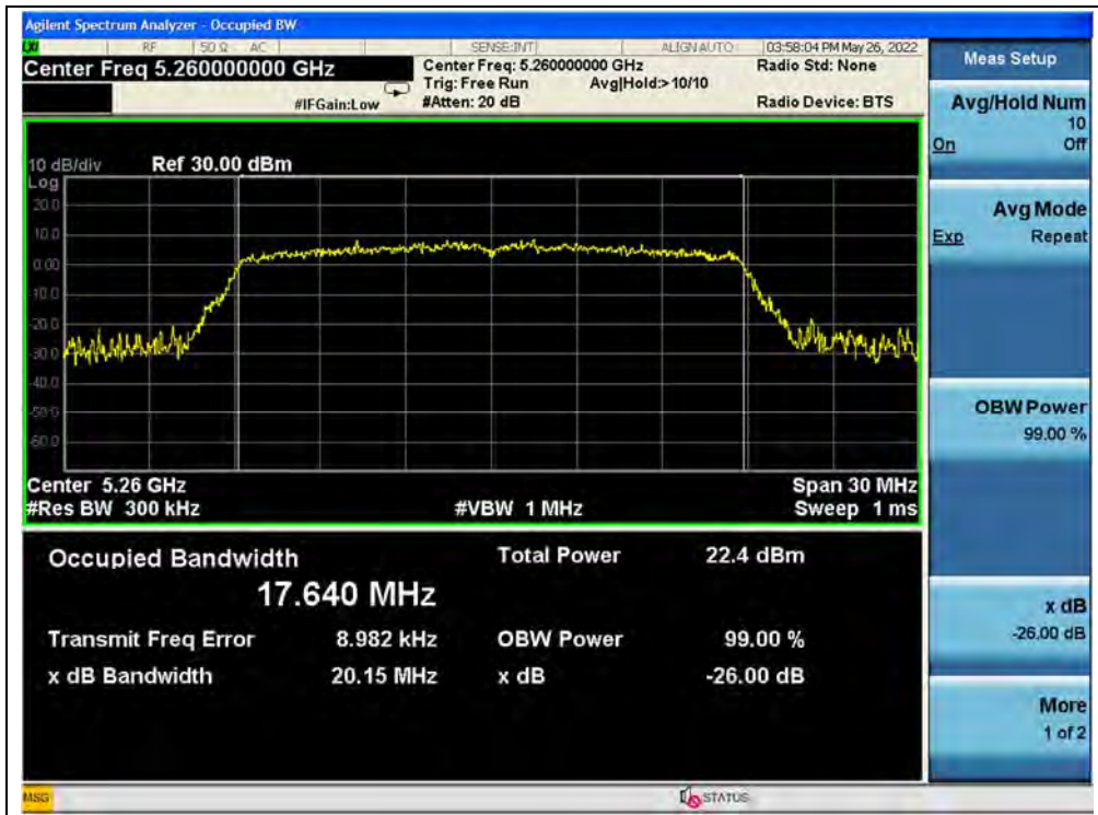
(Channel 52, 5260MHz, 802.11ac (VHT20))
