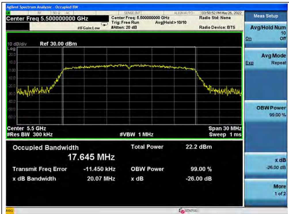
(Channel 100, 5500MHz, 802.11ac (VHT20))
