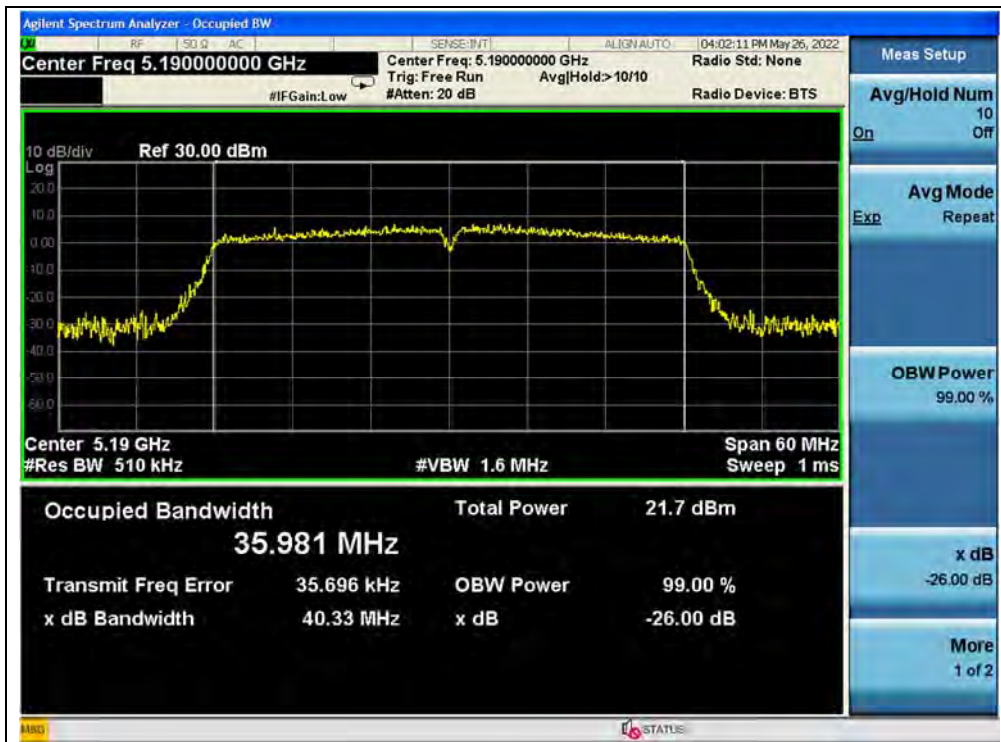
(Channel 38, 5190MHz, 802.11ac (VHT40))
