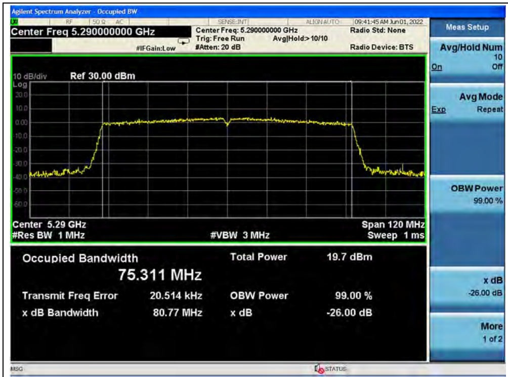
(Channel 58, 5290MHz, 802.11ac (VHT80))
