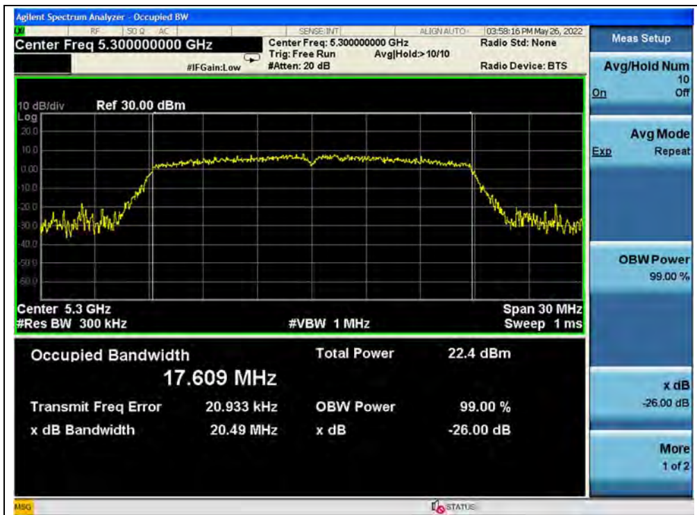
(Channel 60, 5300MHz, 802.11ac (VHT20))
