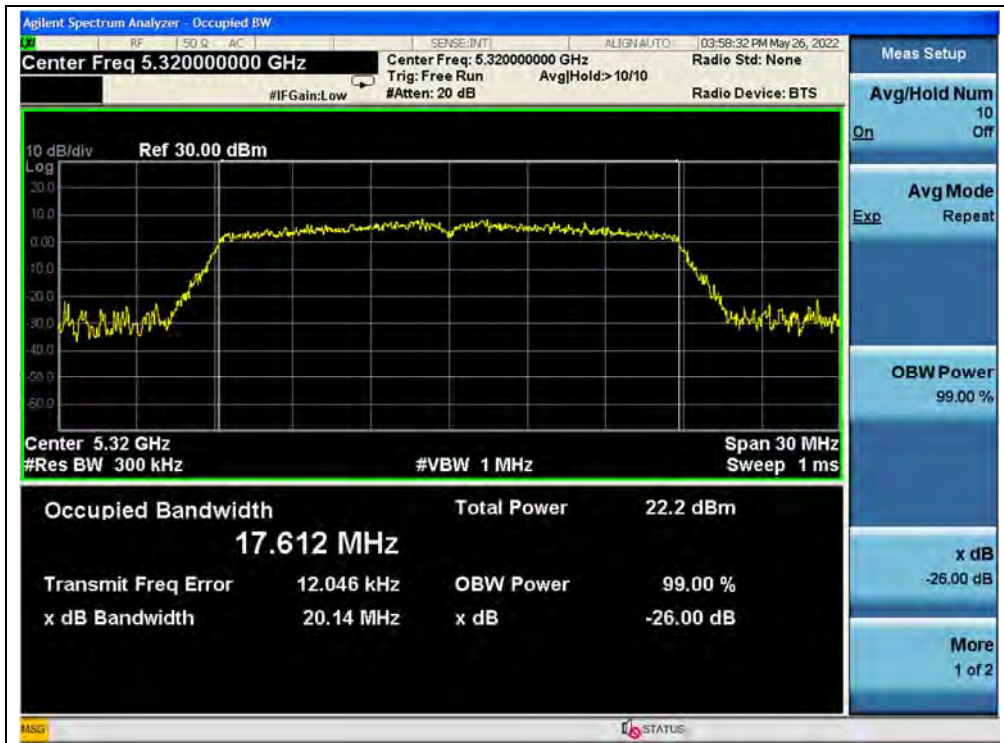
(Channel 64, 5320MHz, 802.11ac (VHT20))
