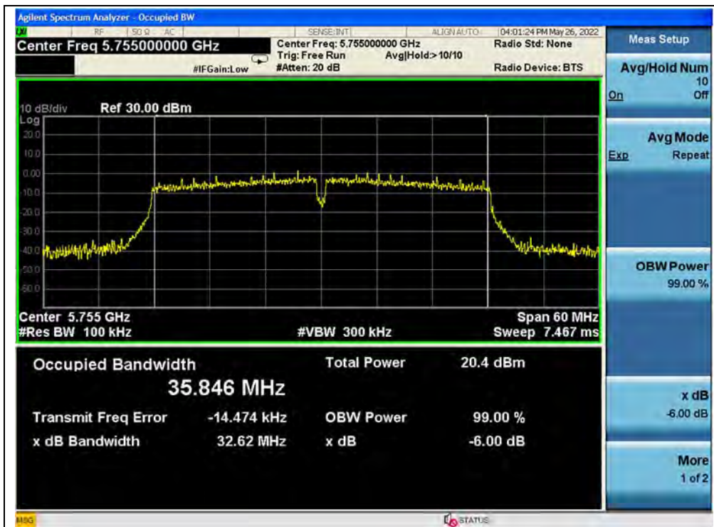
(Channel 151, 5755MHz, 802.11ac (VHT40))
