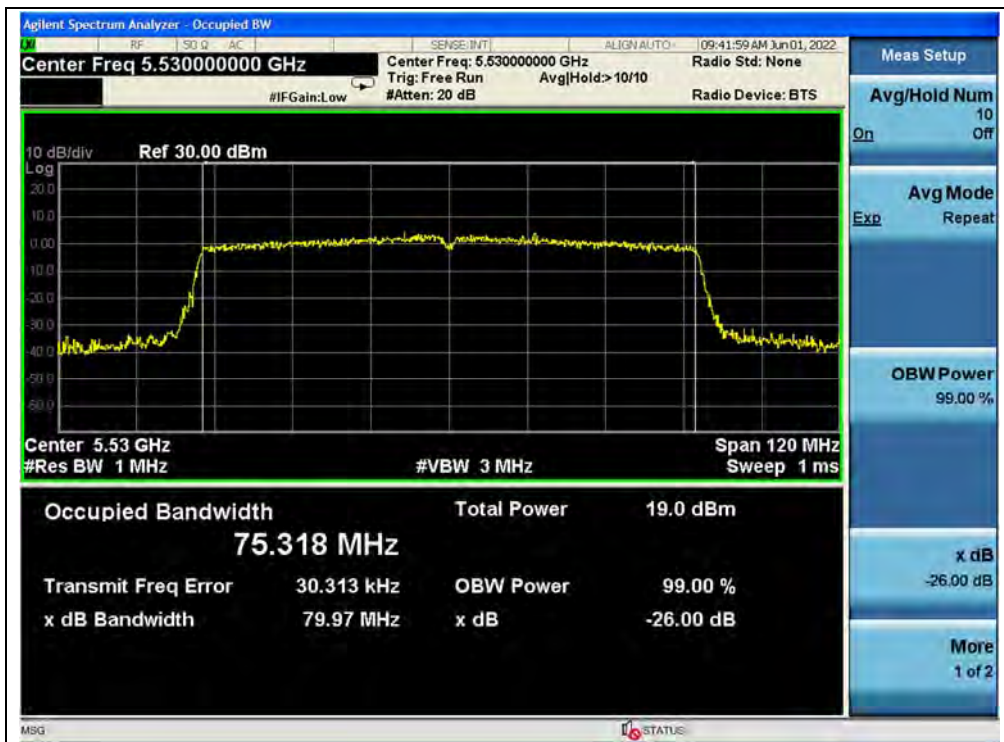
(Channel 106, 5530MHz, 802.11ac (VHT80))
