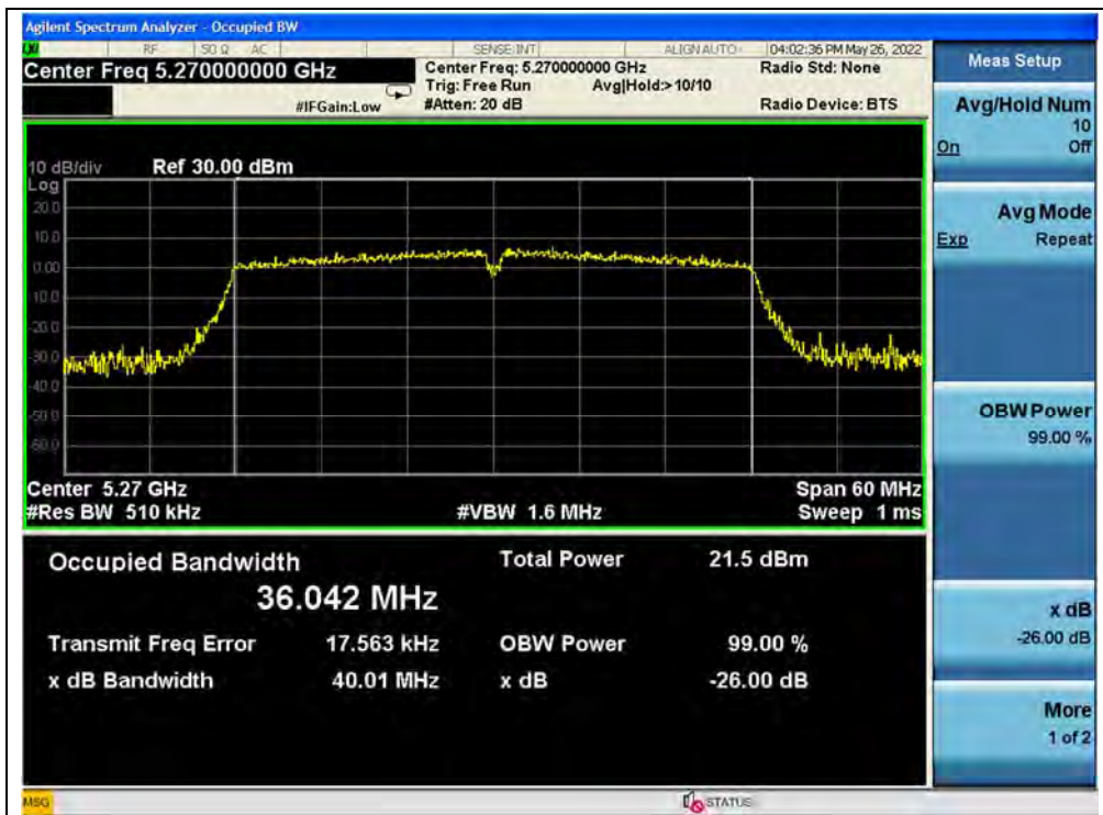
(Channel 54, 5270MHz, 802.11ac (VHT40))
