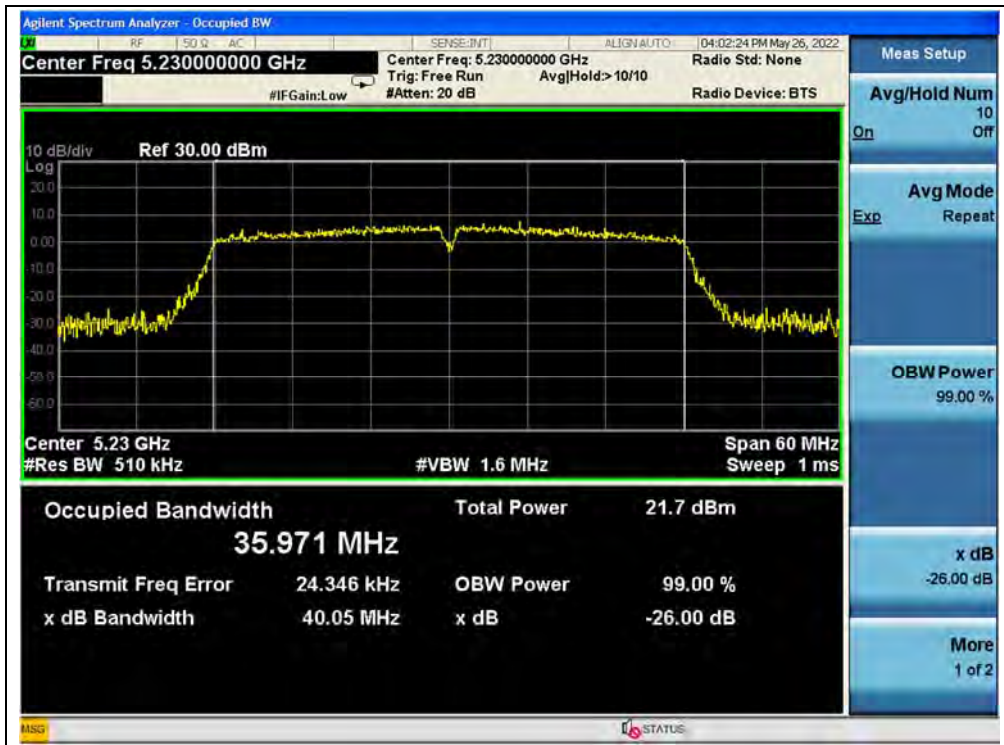
(Channel 46, 5230MHz, 802.11ac (VHT40))
