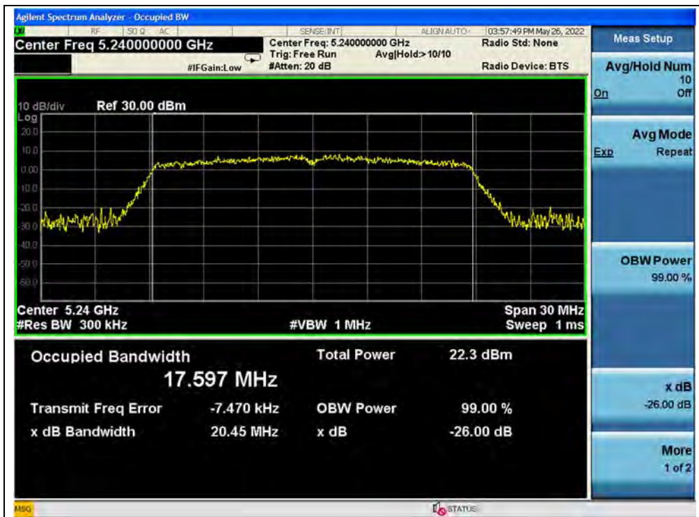
(Channel 48, 5240MHz, 802.11ac (VHT20))
