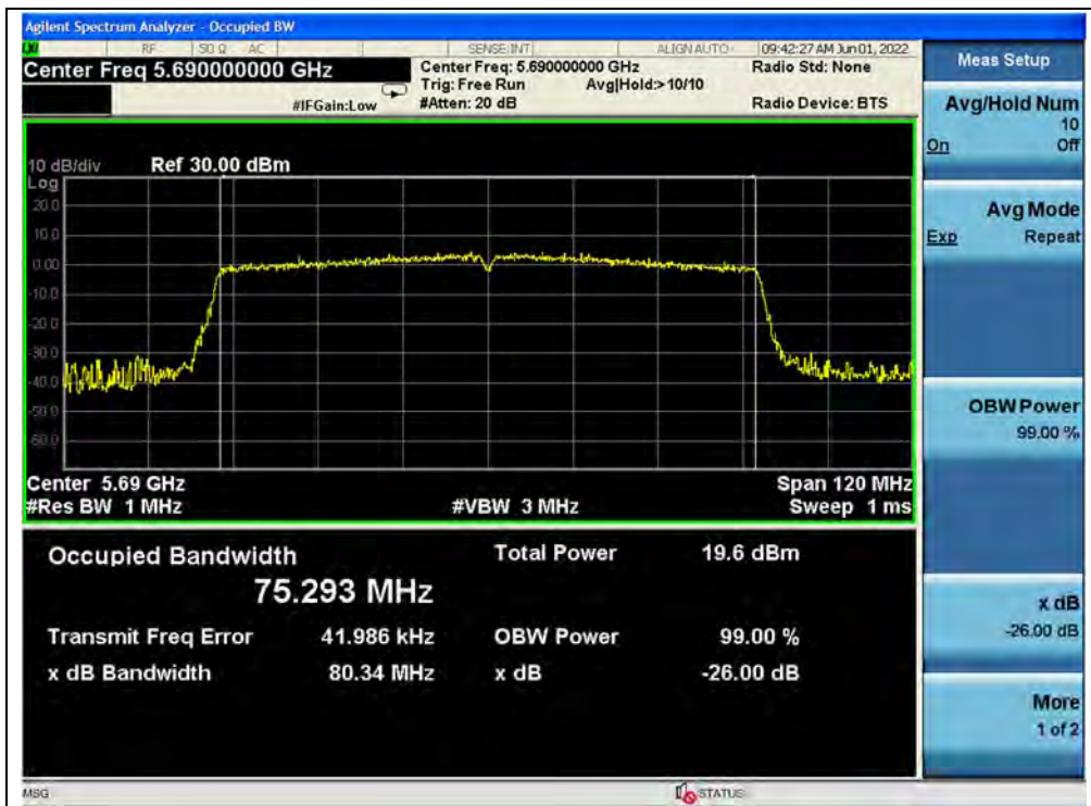
(Channel 138, 5690MHz, 802.11ac (VHT80))
