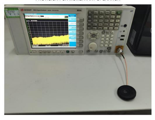
FCC RADIATED EMISSION TEST SETUP
