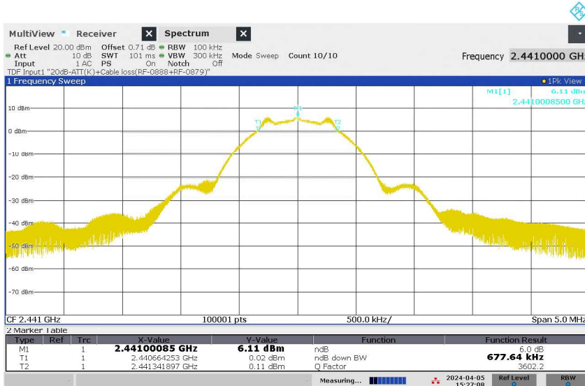
Figure 3: 6dB Bandwidth, Original Wireless Communication, Mode M (2441MHz), ANT1
