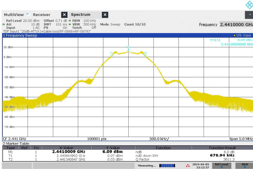
Figure 6: 6dB Bandwidth, Original Wireless Communication, Mode M (2441MHz), ANT2
