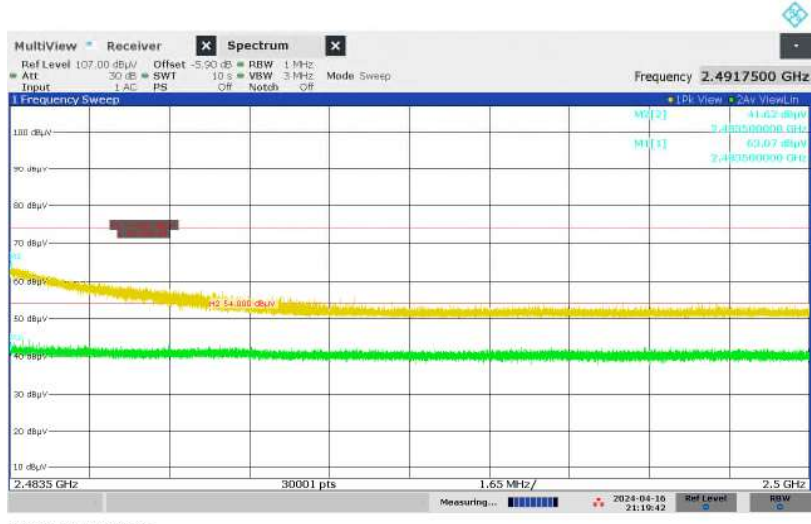
Figure 61: Restricted-band Band-edge, Spectral Diagram, Original Wireless Communication (2480MHz, ANT2) + WLAN 2.4GHz, Vertical Antenna Orientation
