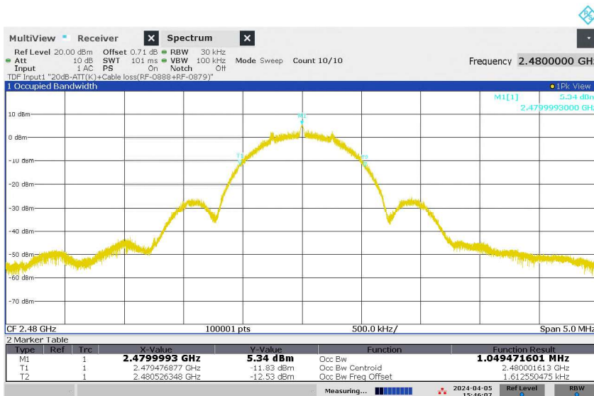
Figure 10: 99% Bandwidth, Original Wireless Communication, Mode H (2480MHz), ANT1
