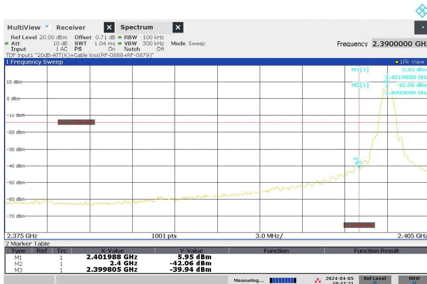
Figure 17: Authorized-band band-edge, Original Wireless Communication, Mode L (2402MHz), ANT 1
