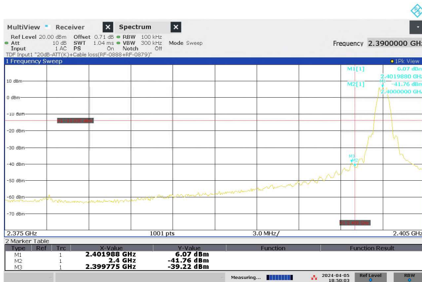
Figure 22: Authorized-band band-edge, Original Wireless Communication, Mode L (2402MHz), ANT 2
