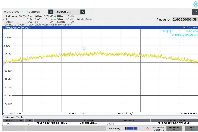
Figure 27: Power Spectral Density, Original Wireless Communication, Mode L (2402MHz), ANT2
