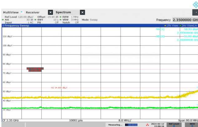
Figure 50: Restricted-band Band-edge, Spectral Diagram, Original Wireless Communication (2402MHz, ANT2) + WLAN 5GHz + Bluetooth Low Energy, Horizontal Antenna Orientation
