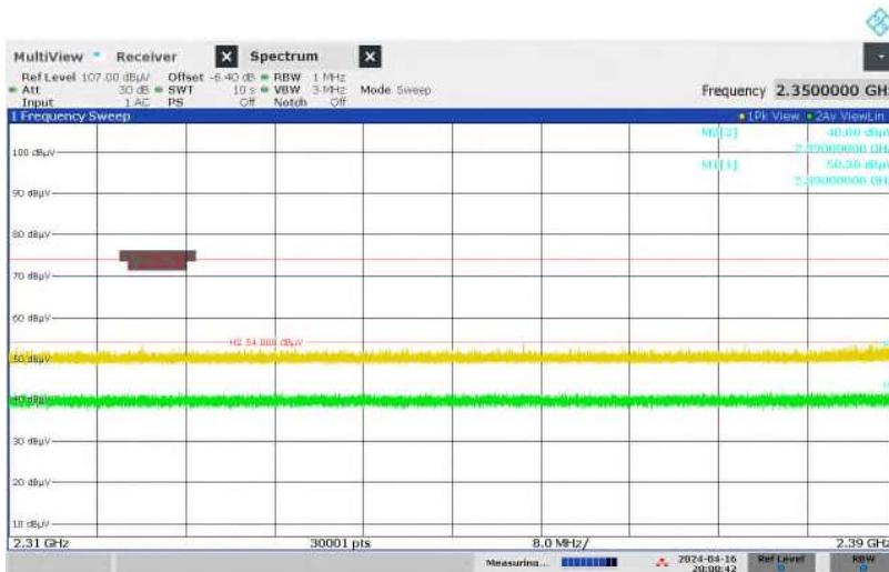
Figure 58: Restricted-band Band-edge, Spectral Diagram, Original Wireless Communication (2402MHz, ANT2) + WLAN 2.4GHz, Horizontal Antenna Orientation
