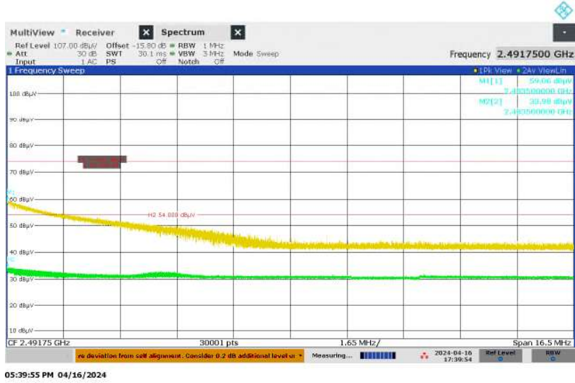
Figure 33: Restricted-band Band-edge, Spectral Diagram, Original Wireless Communication, 2480MHz, Vertical Antenna Orientation, ANT1
