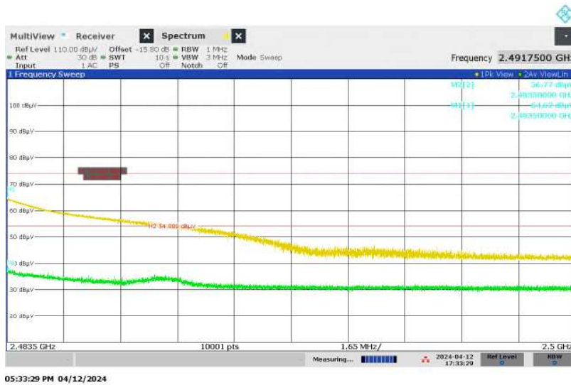
Figure 36: Restricted-band Band-edge, Spectral Diagram, Original Wireless Communication, 2480MHz, Horizontal Antenna Orientation, ANT2
