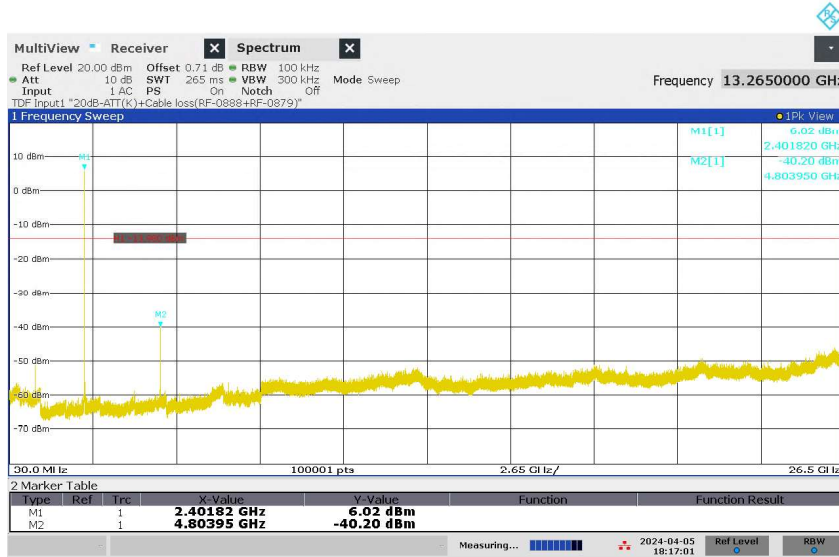
Figure 14: Conducted Spurious Emissions, 30MHz - 25GHz, Original Wireless Communication, Mode L (2402MHz), ANT 1
