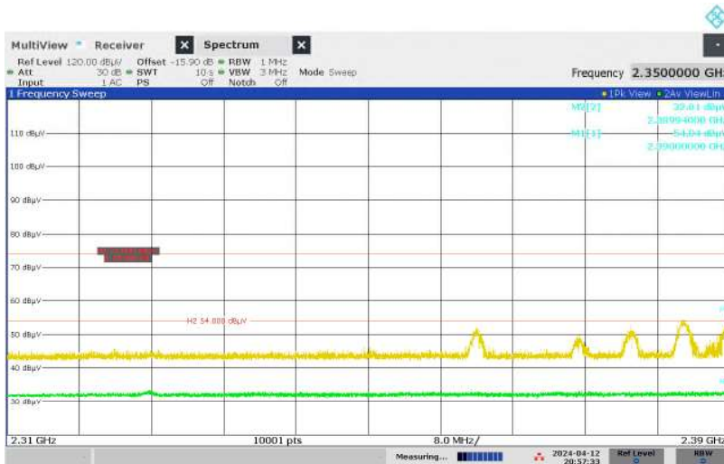
Figure 42: Restricted-band Band-edge, Spectral Diagram, Original Wireless Communication (2402MHz, ANT2) + WLAN 5GHz + Bluetooth Classic, Horizontal Antenna Orientation
