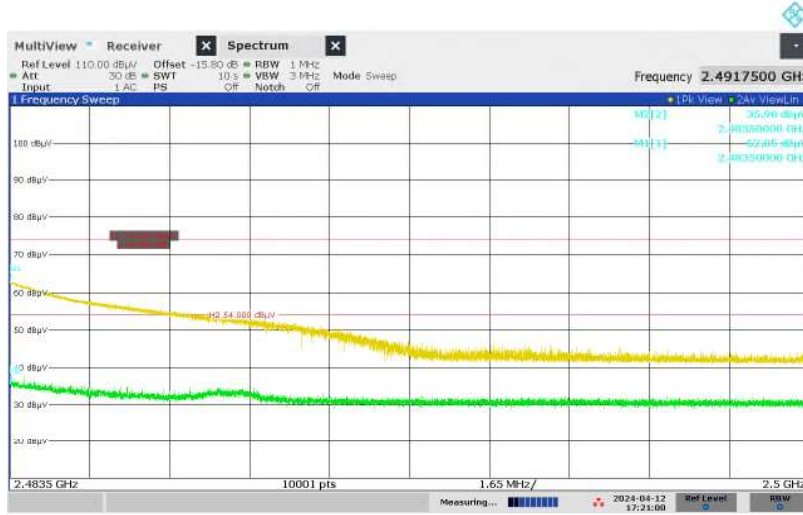
Figure 37: Restricted-band Band-edge, Spectral Diagram, Original Wireless Communication, 2480MHz, Vertical Antenna Orientation, ANT2
