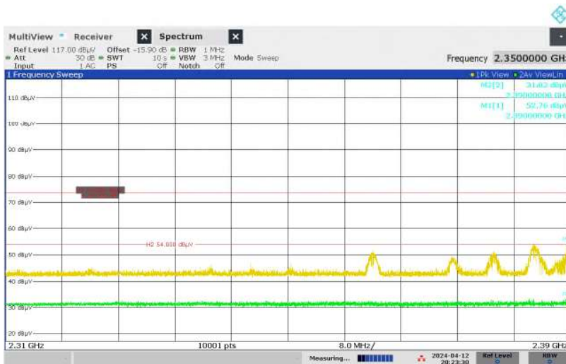
Figure 38: Restricted-band Band-edge, Spectral Diagram, Original Wireless Communication (2402MHz, ANT1) + WLAN 5GHz + Bluetooth Classic, Horizontal Antenna Orientation
