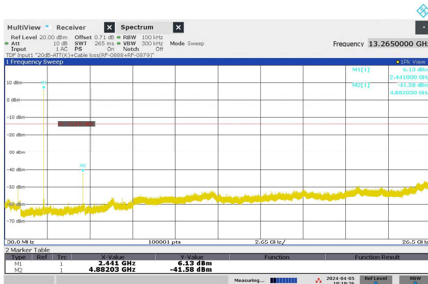
Figure 15: Conducted Spurious Emissions, 30MHz - 25GHz, Original Wireless Communication, Mode M (2441MHz), ANT 1
