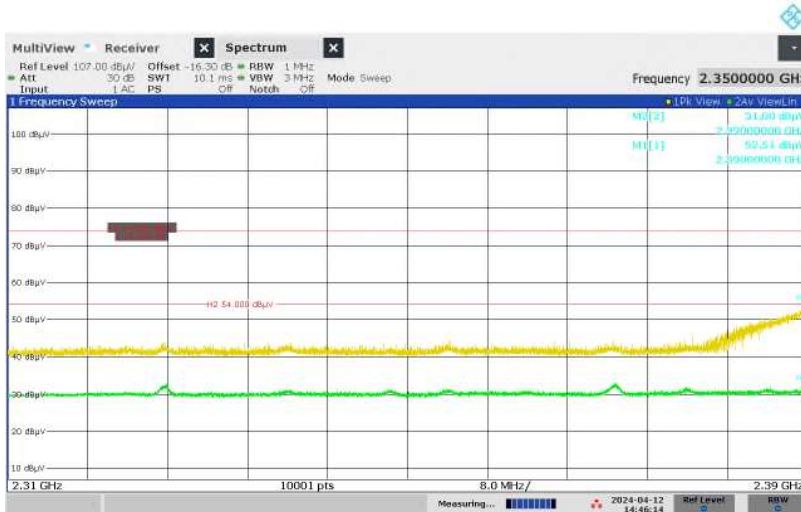
Figure 34: Restricted-band Band-edge, Spectral Diagram, Original Wireless Communication, 2402MHz, Horizontal Antenna Orientation, ANT2
