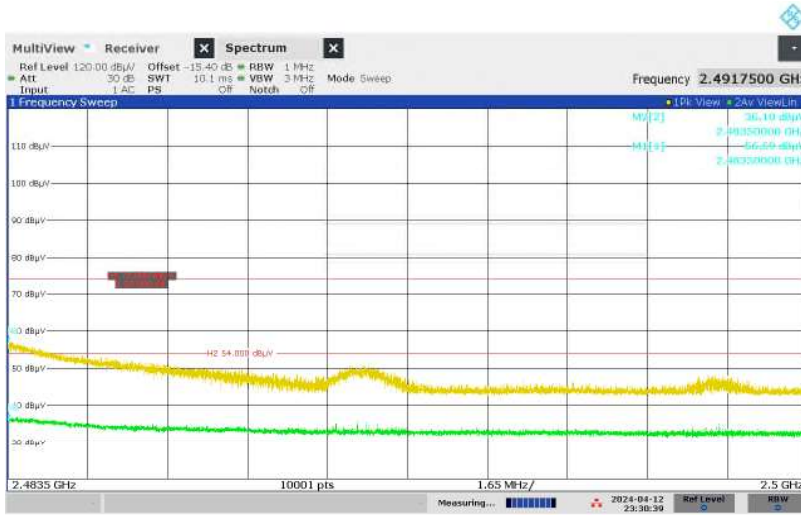
Figure 41: Restricted-band Band-edge, Spectral Diagram, Original Wireless Communication (2480MHz, ANT1) + WLAN 5GHz + Bluetooth Classic, Vertical Antenna Orientation
