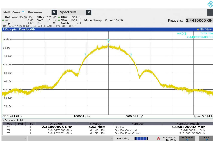
Figure 12: 99% Bandwidth, Original Wireless Communication, Mode M (2441MHz), ANT2
