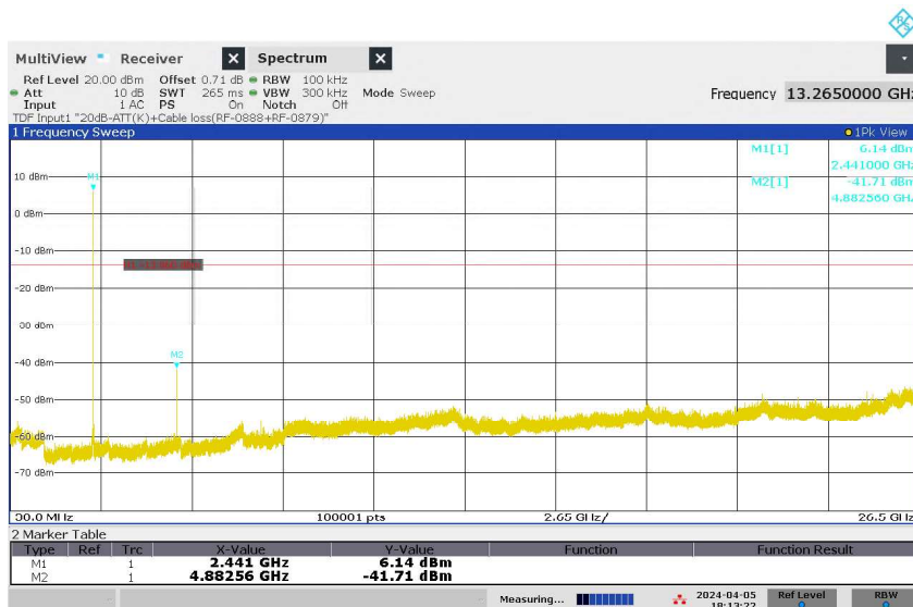
Figure 20: Conducted Spurious Emissions, 30MHz - 25GHz, Original Wireless Communication, Mode M (2441MHz), ANT 2
