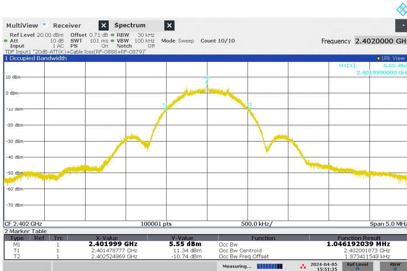
Figure 8: 99% Bandwidth, Original Wireless Communication, Mode L (2402MHz), ANT1
