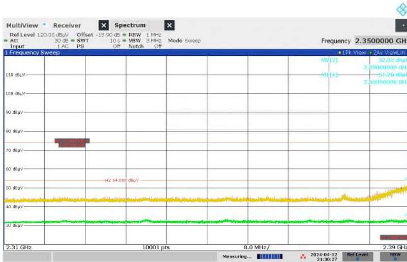
Figure 46: Restricted-band Band-edge, Spectral Diagram, Original Wireless Communication (2402MHz, ANT1) + WLAN 5GHz + Bluetooth Low Energy, Horizontal Antenna Orientation
