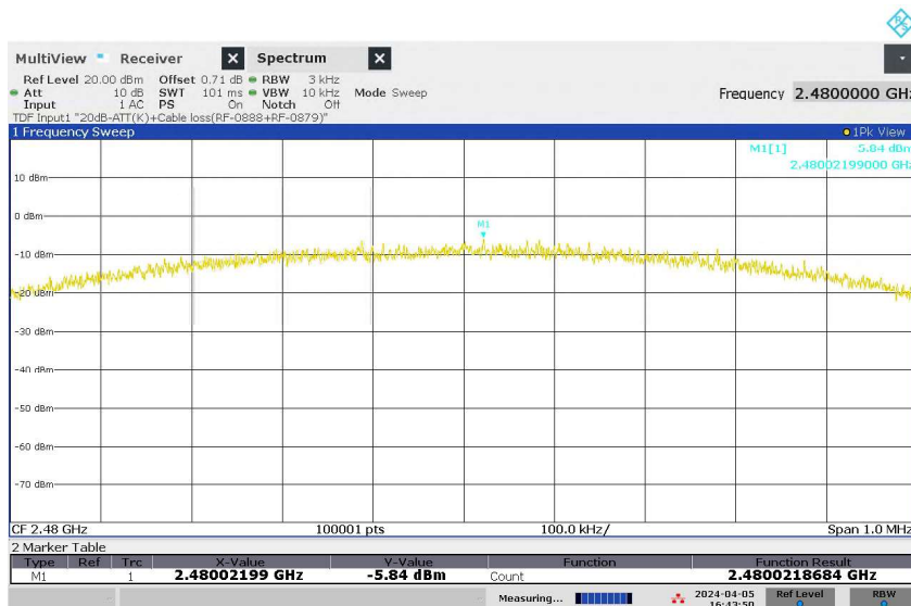
Figure 29: Power Spectral Density, Original Wireless Communication, Mode H (2480MHz), ANT2
