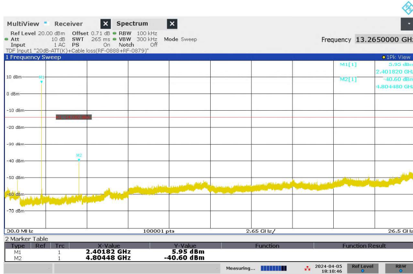
Figure 19: Conducted Spurious Emissions, 30MHz - 25GHz, Original Wireless Communication, Mode L (2402MHz), ANT 2
