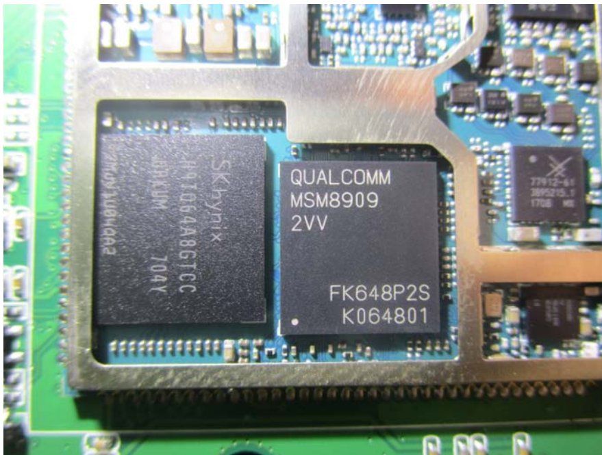
EUT -2G&3G&4G Chip View
