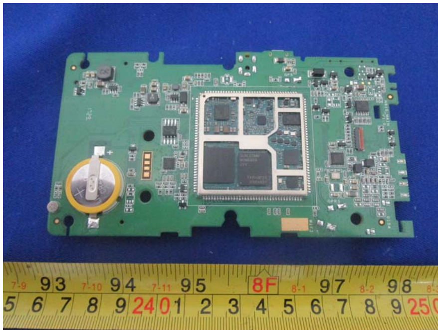
EUT – Main Board Unshielded Bottom View
