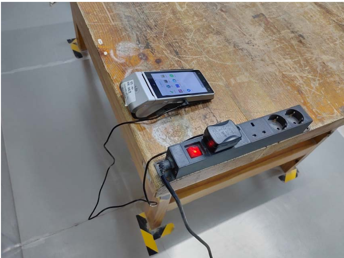
Conducted Emissions Side View
