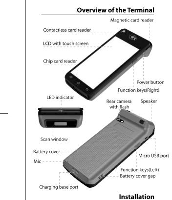
The terminal should be kept away from very hot zone and protected from vibrations, dust, damp or
