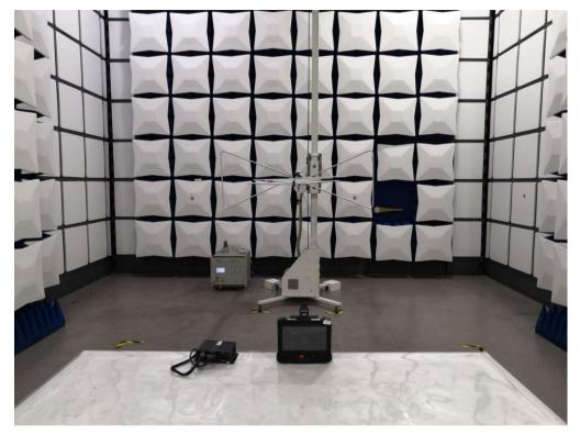
RADIATED EMISSION ABOVE 1G TEST SETUP
