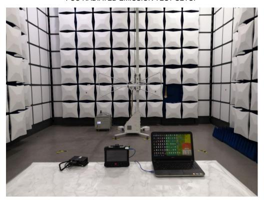
FCC RADIATED EMISSION TEST SETUP
