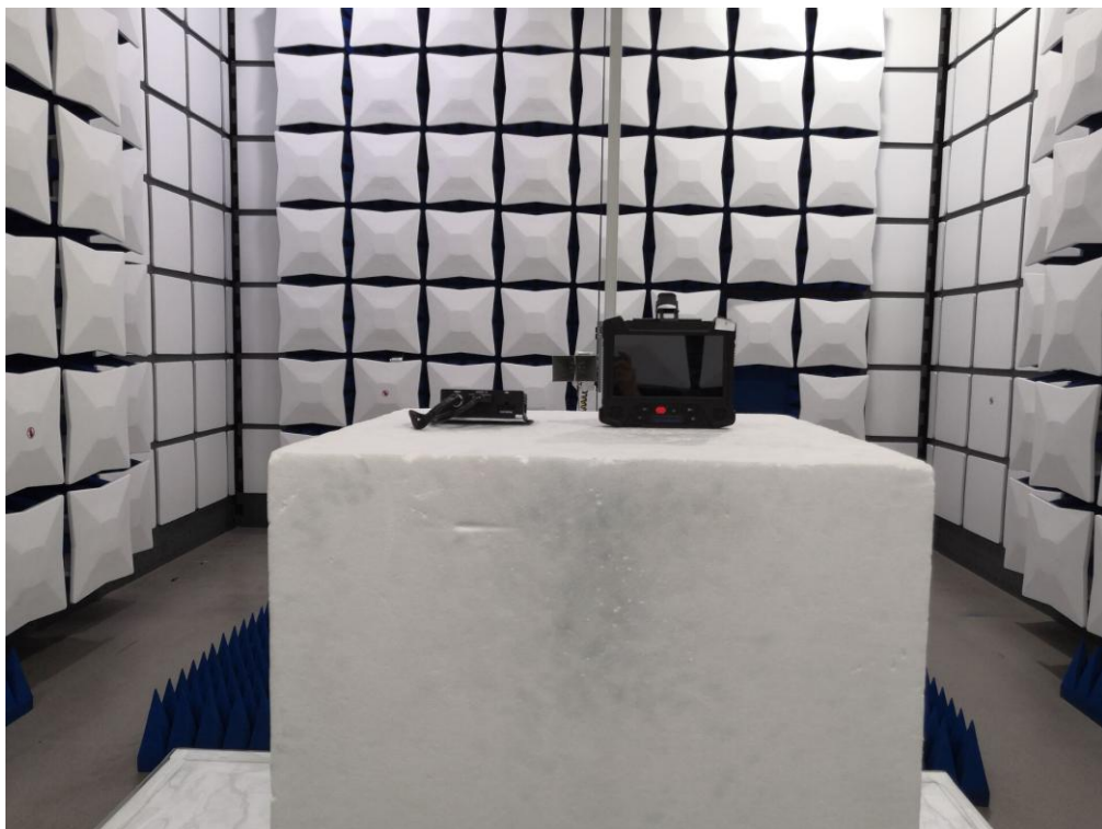
RADIATED EMISSION ABOVE 1G TEST SETUP
