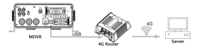
The 4G router mainly works with Mobile DVR. When there is no built-in network communication module in the Mobile DVR, user can connect the USB interface at the rear panel of MDVR to the one of wireless 4G router to realize the long-distance audio & video data transmission of MDVR through 4G wireless network.
