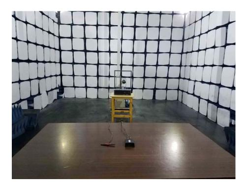
Spurious Radiation Test Setup (30MHz to 1G)
