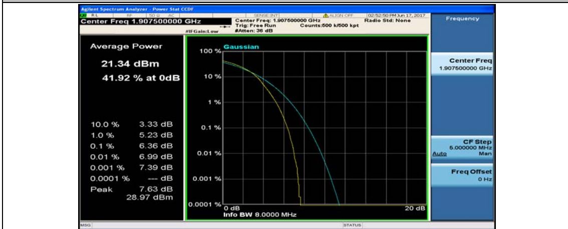
(Channel Bandwidth:15 MHz)_HCH_16QAM_75RB#0
