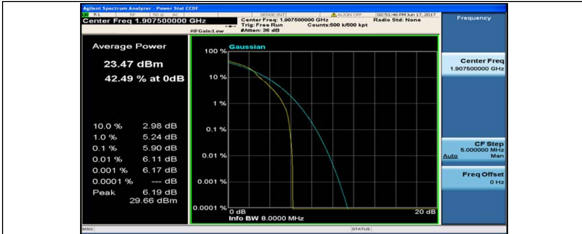
(Channel Bandwidth:15 MHz)_HCH_16QAM_1RB#74
