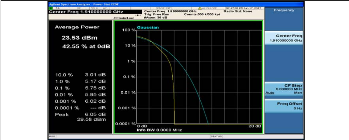
Channel Bandwidth: 10 MHz_HCH_16QAM_1RB#49
