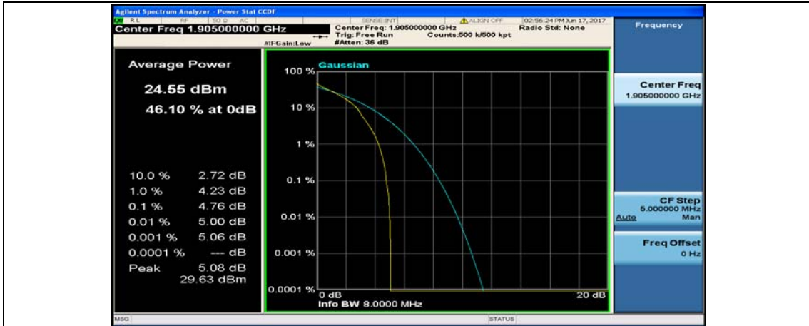
(Channel Bandwidth:20 MHz)_HCH_QPSK_1RB#99
