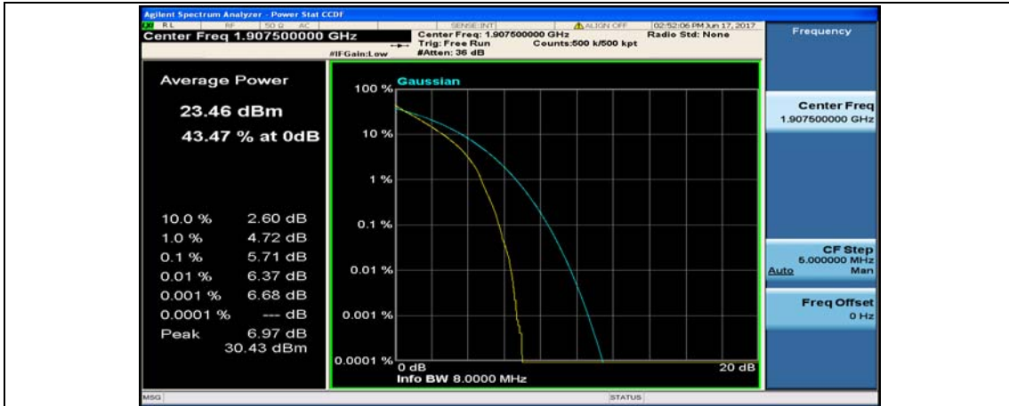
(Channel Bandwidth:15 MHz)_HCH_QPSK_37RB#38
