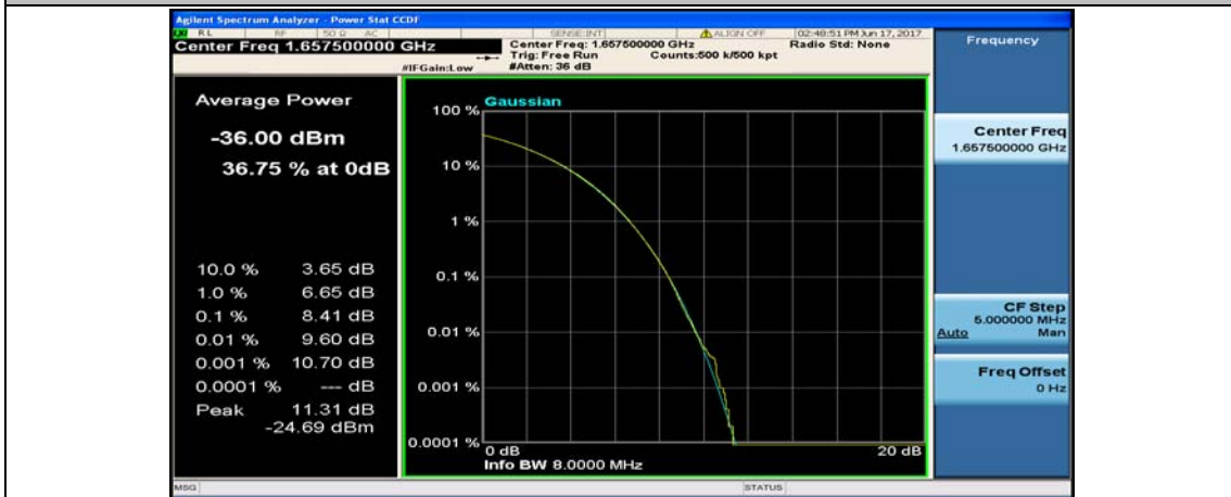
(Channel Bandwidth:15 MHz)_LCH_QPSK_37RB#38
