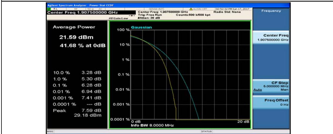
(Channel Bandwidth:15 MHz)_HCH_16QAM_75RB#0
