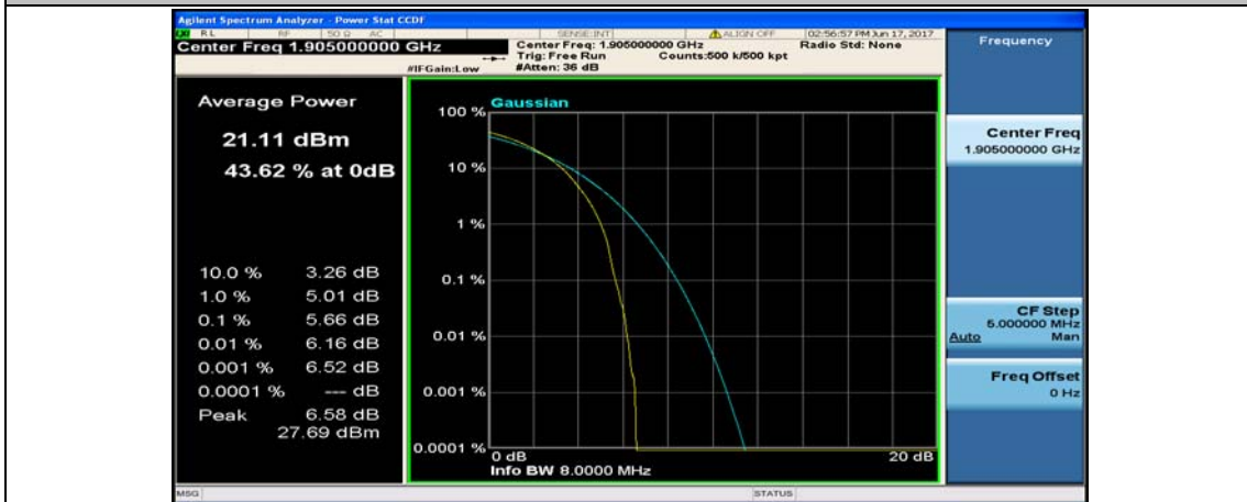
(Channel Bandwidth:20 MHz)_HCH_QPSK_50RB#25
