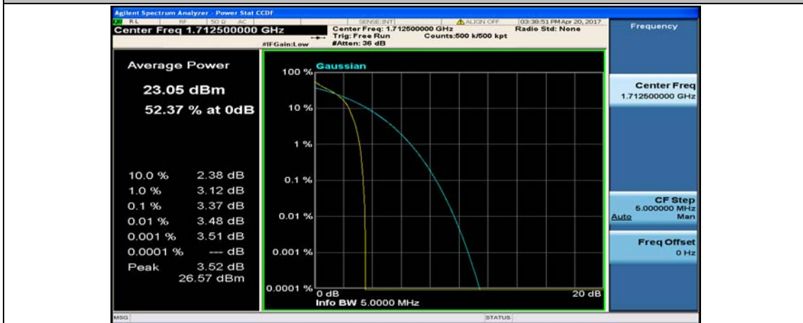
(Channel Bandwidth: 5 MHz)_LCH_QPSK_12RB#0
