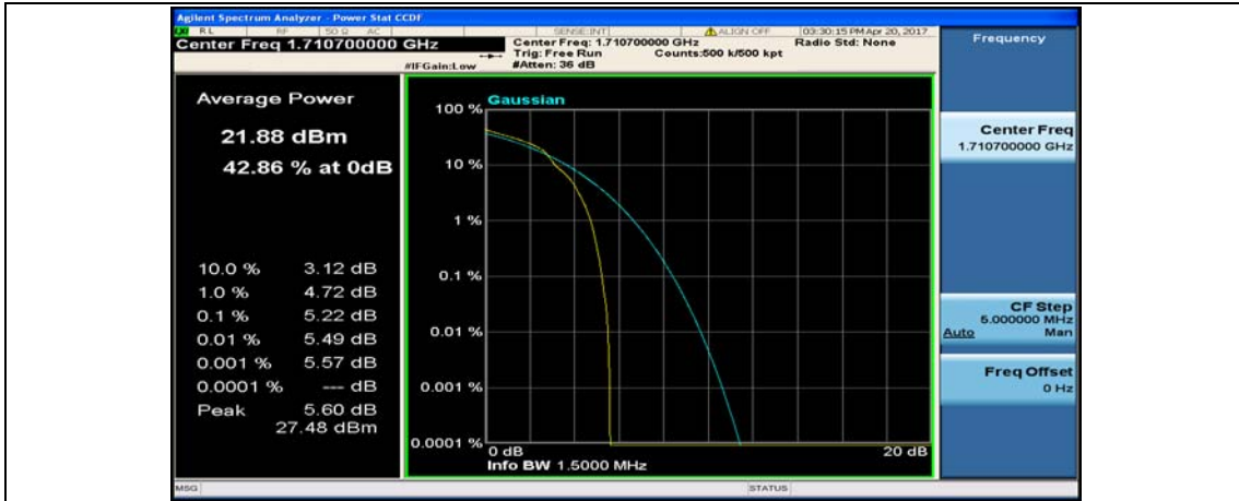
(Channel Bandwidth: 1.4 MHz)_LCH_16QAM_1RB#3
