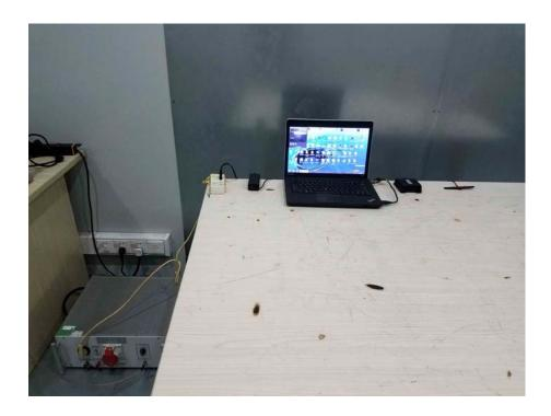
Radiation Emission Test Setup (30MHz to 1GHz)
