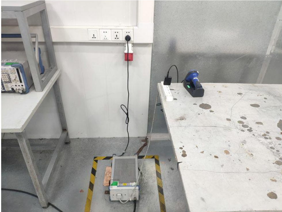
Photo of Power Line Conducted Emission Test
