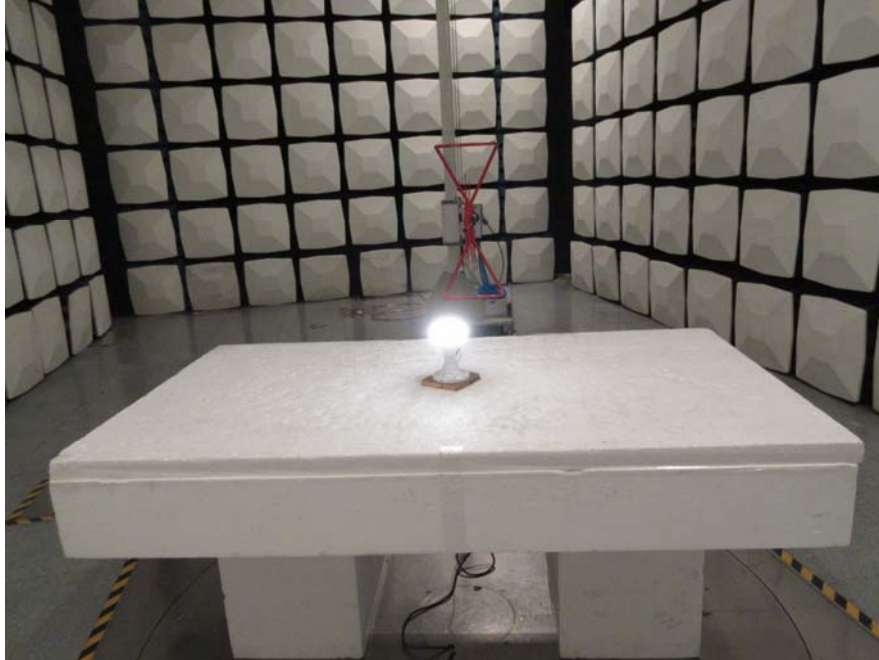
Radiated Emission View (Below 1 GHz)
