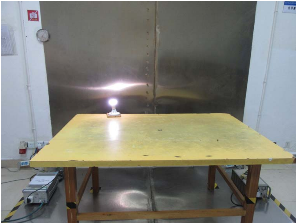
Conducted Emission Front View
