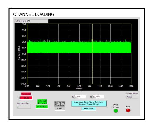
The level of traffic loading on the channel by the EUT is 33.55%
