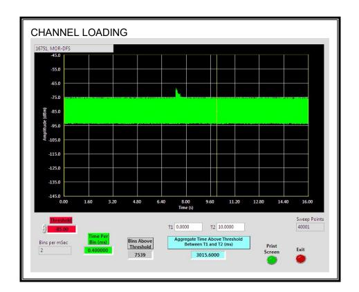
The level of traffic loading on the channel by the EUT is 30.16%
