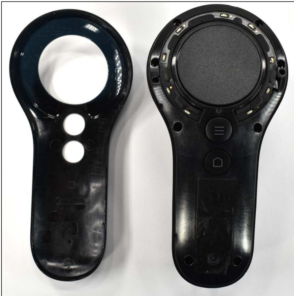
Figure 1: Controller – first layer below the top cover
