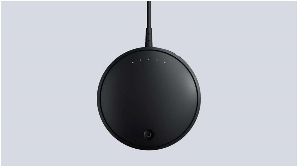
*The five lights towards the top of the Compute Pack will be illuminated when fully powered.*
