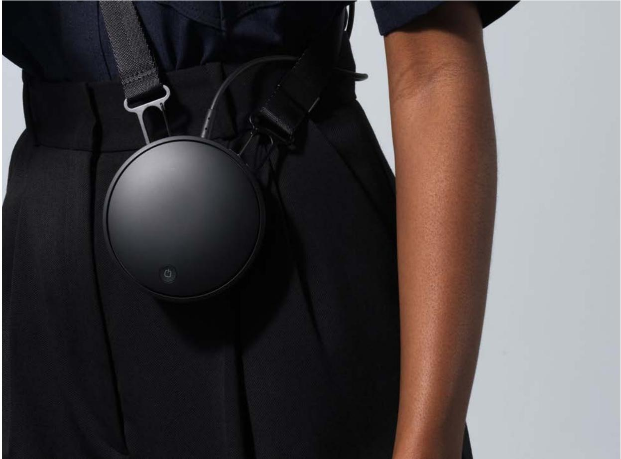
*Fasten the carabiners on the ends of the Shoulder Strap to the Compute Pack to hold it into place.*
