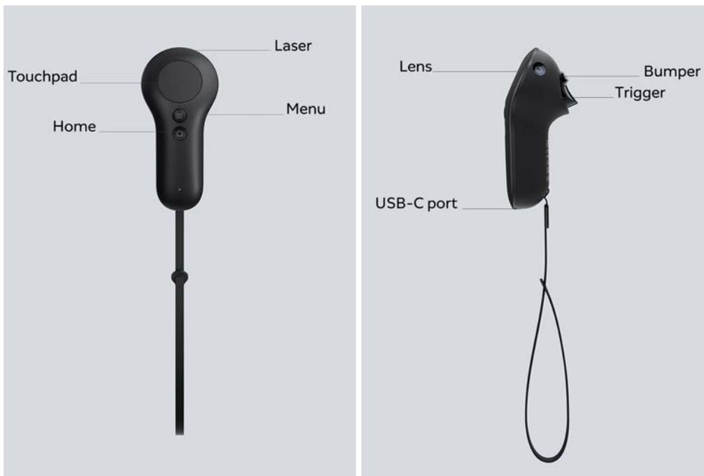
*Identify the buttons and controls on the Magic Leap 2 Controller and Compute Pack pictured.*
