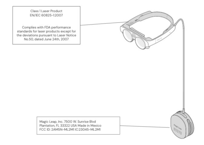
The Manufacturer Identification label is located on the back of the Compute Pack clip. Turn the Compute Pack over to see it. It reads as follows:
