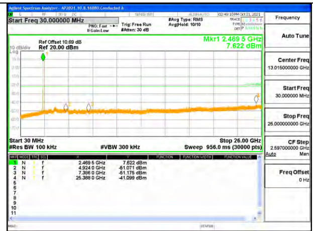
OUT-OF-BAND HIGH CHANNEL 11 ANTENNA 2
