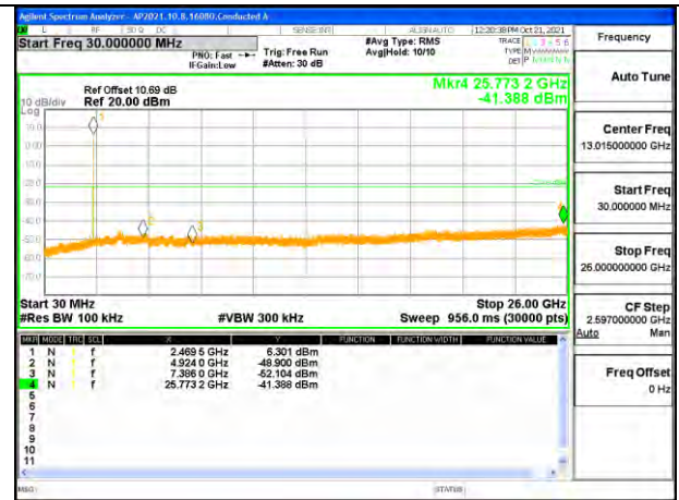
OUT-OF-BAND HIGH CHANNEL 11 ANTENNA 1
