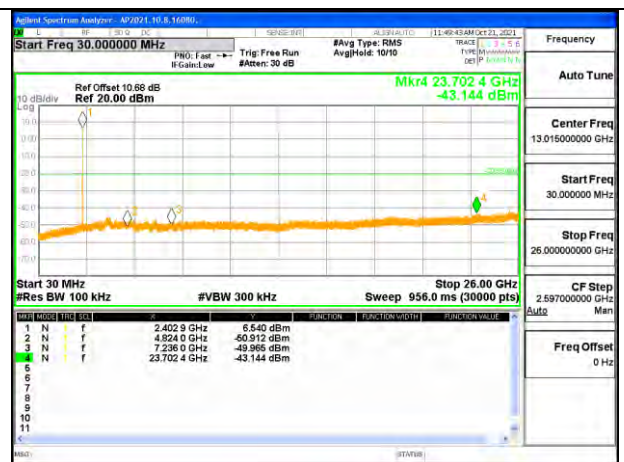
OUT-OF-BAND LOW CHANNEL 1 ANTENNA 1
