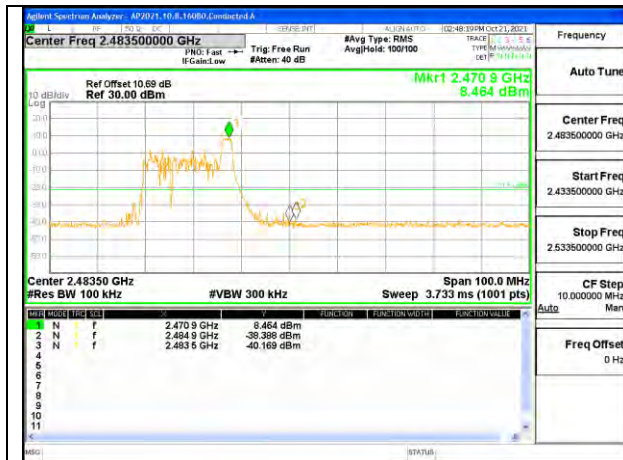
HIGH CHANNEL 11 BANDEDGE ANTENNA 2
