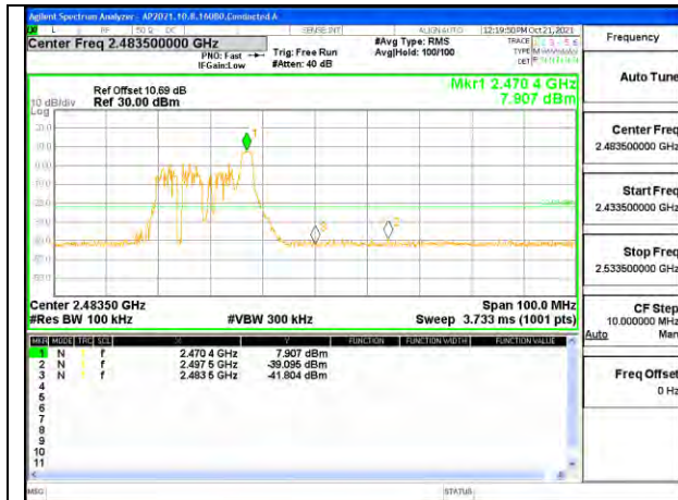
HIGH CHANNEL 11 BANDEDGE ANTENNA 1
