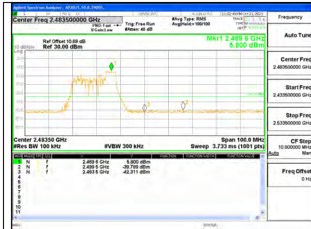
HIGH CHANNEL 11 BANDEDGE ANTENNA 1
