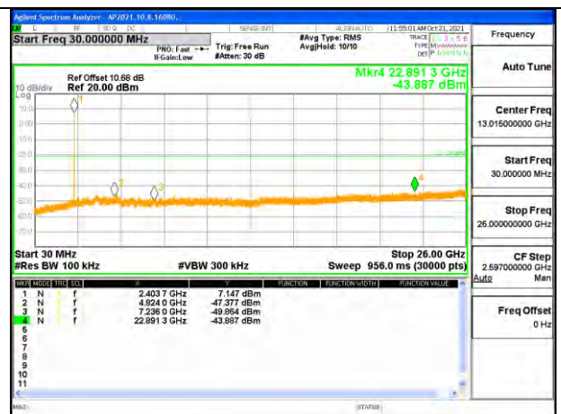
OUT-OF-BAND LOW CHANNEL 1 ANTENNA 2
