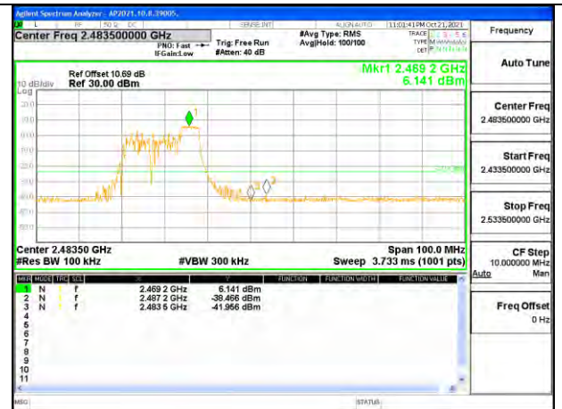
HIGH CHANNEL 11 BANDEDGE ANTENNA 1
