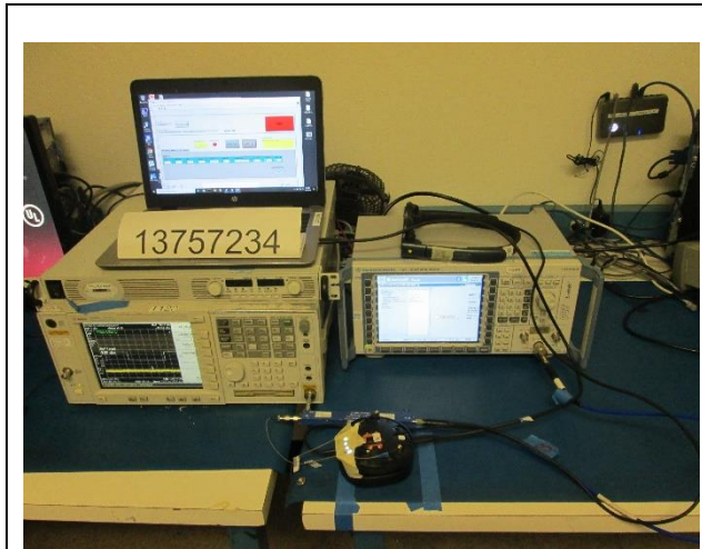
RF ANTENNA PORT CONDUCTED
