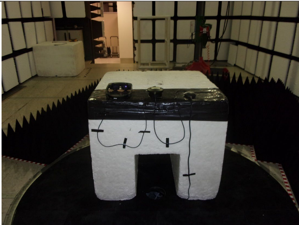
Photo of test setup for Radiated Emissions: 1 GHz - 18 GHz, Wearpack + ML-2 Charger, Flat, Rear
