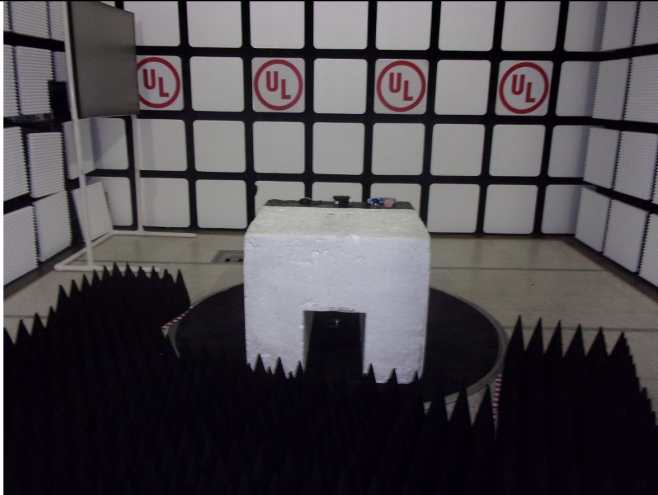
Photo of test setup for Radiated Emissions: 1 GHz - 18 GHz, Wearpack + ML-2 Charger, Flat, Front
