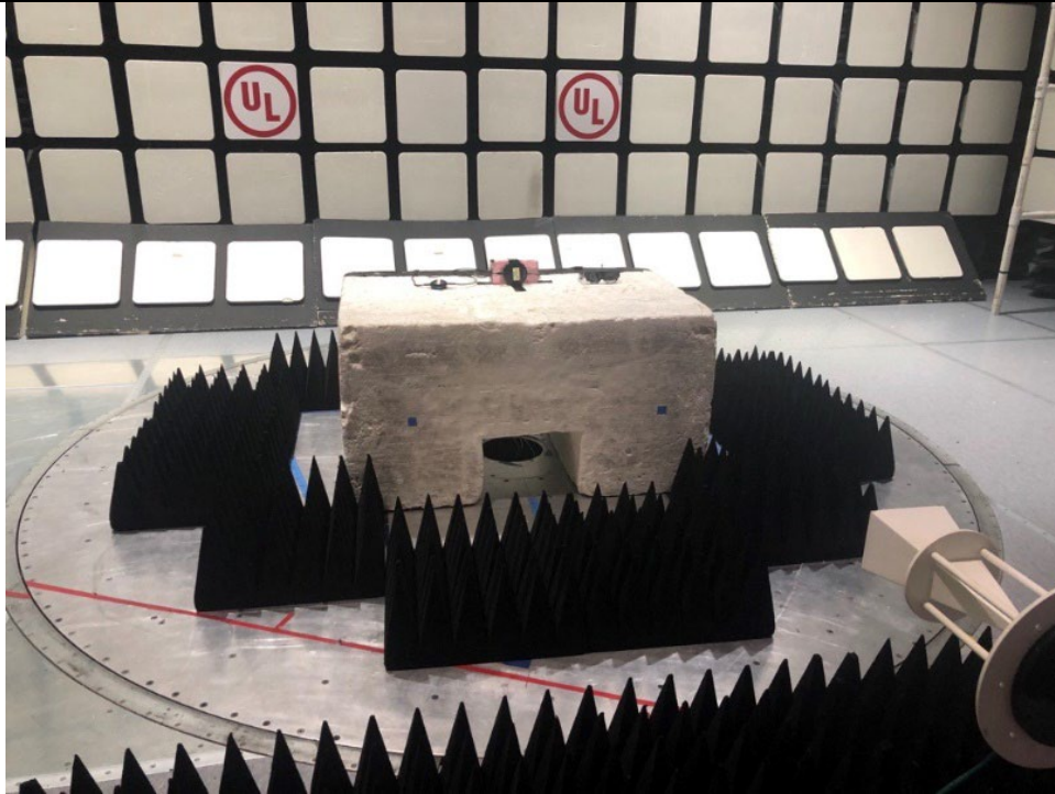
Photo of test setup for Radiated Emissions: 18 GHz - 40 GHz, Wearpack + ML-2 Charger, Horizontal, Rear
