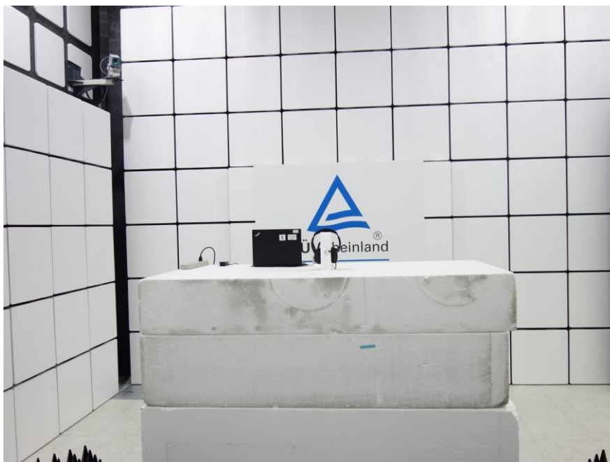
Photograph 2: Set-up for Spurious Emissions (Front View 2)
