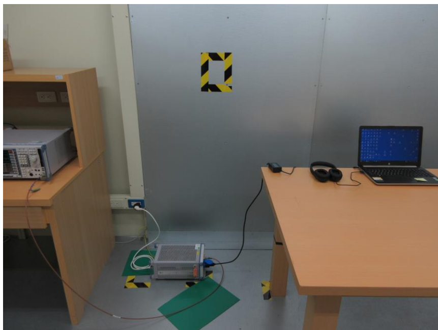
Photograph 6: Set-up for AC Mains (Front View)
