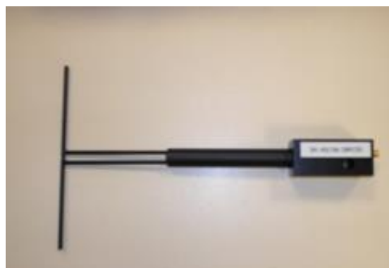
Figure 1 – MVG COMOSAR Validation Dipole
