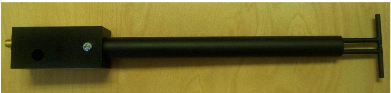
Figure 1 – MVG COMOSAR Validation Dipole
