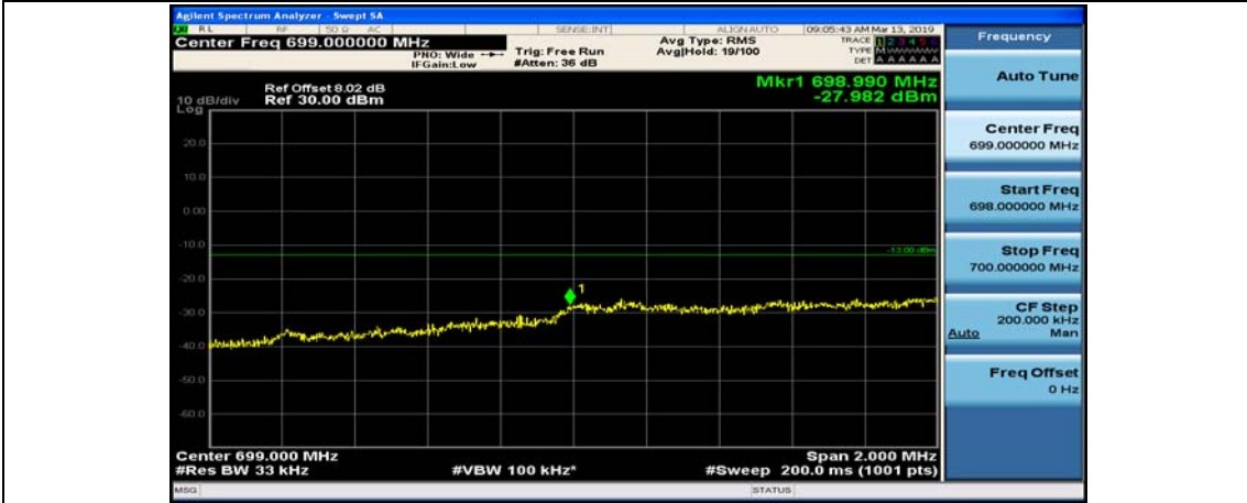
(Channel Bandwidth: 3 MHz)_LCH_QPSK_15RB#0
