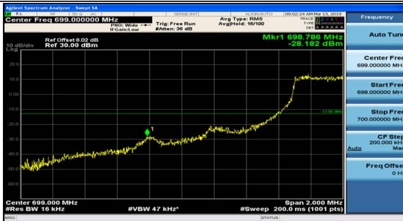
(Channel Bandwidth: 1.4 MHz)_LCH_QPSK_6RB#0
