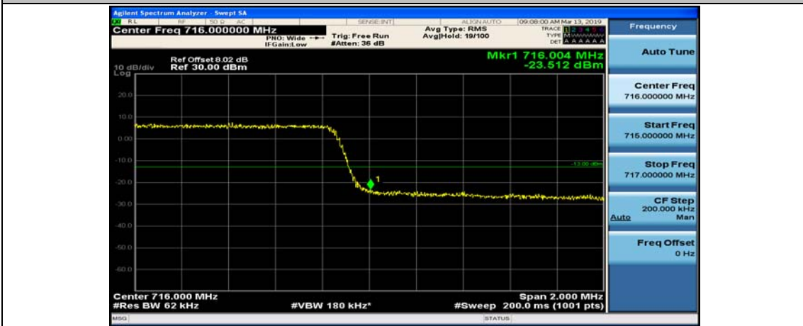
(Channel Bandwidth: 3 MHz)_HCH_16QAM_15RB#0
