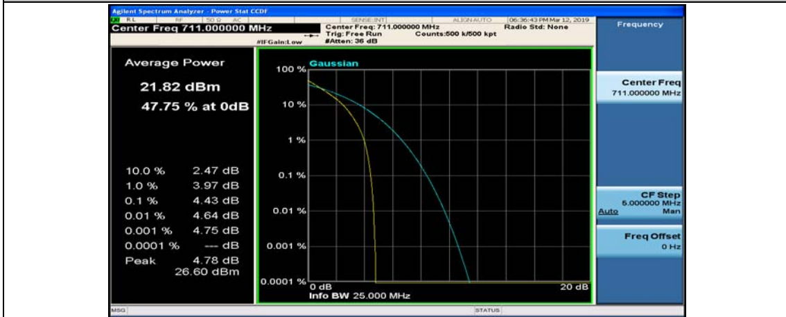
Channel Bandwidth: 10 MHz_HCH_QPSK_25RB#12
