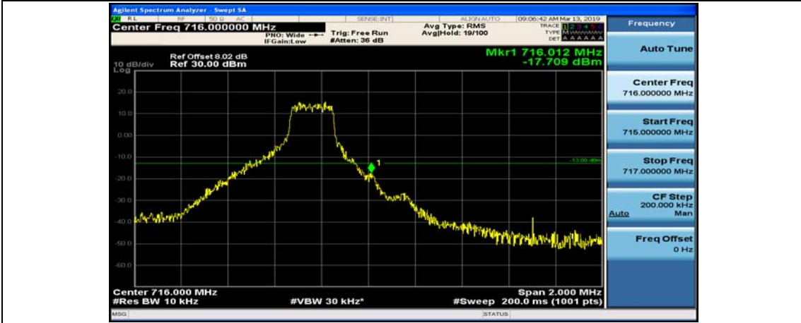
(Channel Bandwidth: 3 MHz)_HCH_QPSK_8RB#0
