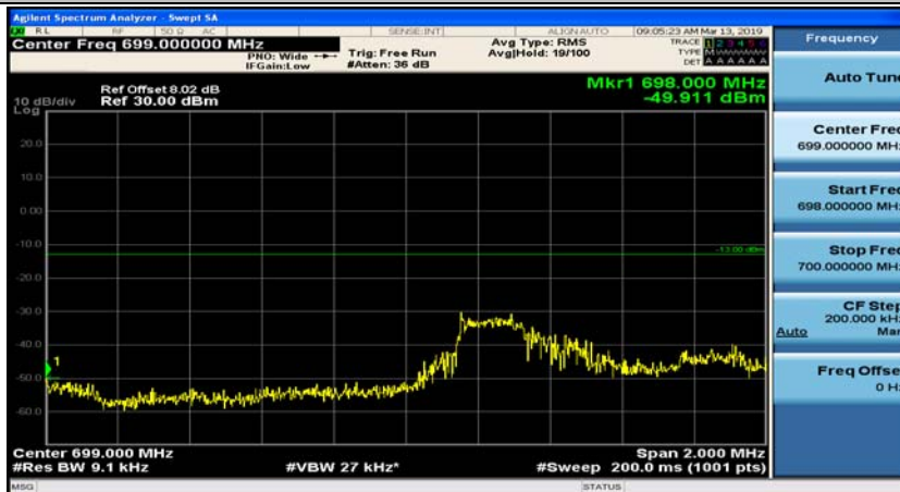
(Channel Bandwidth: 3 MHz)_LCH_16QAM_8RB#0
