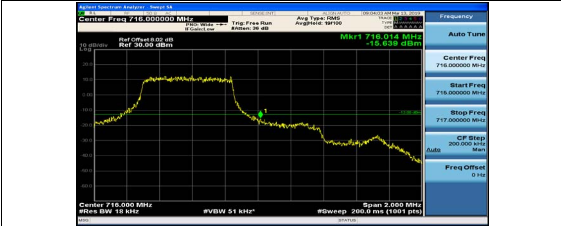
(Channel Bandwidth: 1.4 MHz)_HCH_QPSK_6RB#0
