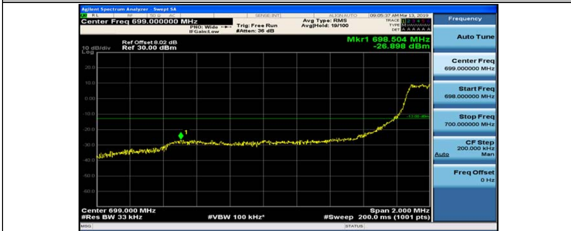
(Channel Bandwidth: 3 MHz)_LCH_QPSK_8RB#7
