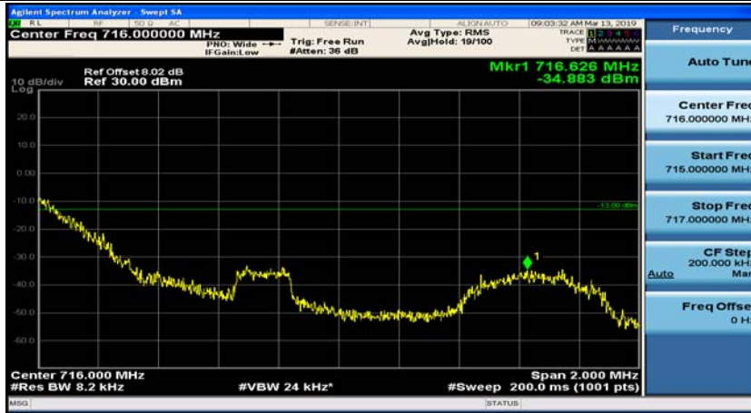
(Channel Bandwidth: 1.4 MHz)_HCH_16QAM_1RB#3
