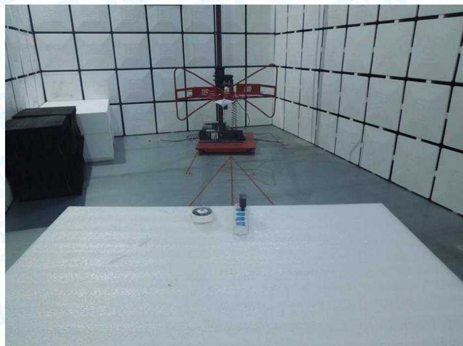
**Photo of Setup for Conducted Emission**
