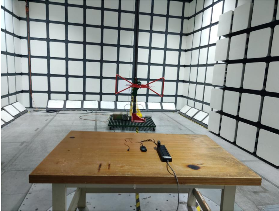
Radiated Emissions View (Below 1 GHz)
