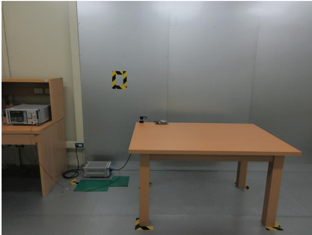
Photograph 15: Set-up for AC Mains (Front View, 37130-AKD3)
