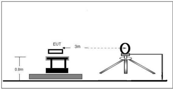
(B) Radiated Emission Test-Up Frequency 30MHz~1GHz
