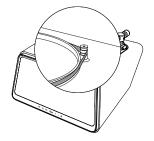
4 Place the drive belt around the sub-platter and motor pulley.
