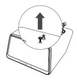
2 Loose the fixing screw and put in a safe place.
