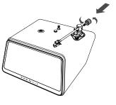
Align the counterweight and the hole, and turn to end.
