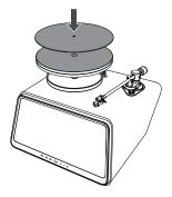
**5** | Place the platter and platter pad in sequence.
