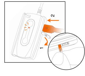
Take off the rubber insert on the side of transmitter You can recharge it through the dual output stock charger, smartphone charger (recommend), laptop computer USB port, or power bank for emergency. Plug the USB side into the port and insert the micro USB head on the transmitter's charging port. The LED indicator will start to flash and it will turn off when fully charged.
