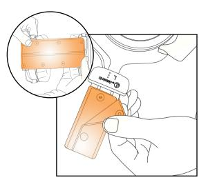
You can take off the head band cushions for cleaning or replace with new one. Hold the edge of the cushion and pull from the first button.
