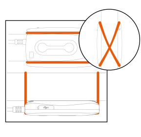
Place the transmitter near the detectors' audio jack on the rod. Wrap the elastic band from the button of rod and hold on the gap of transmitter. If the rod is too thin, twist the elastic band first and follow the above process.
