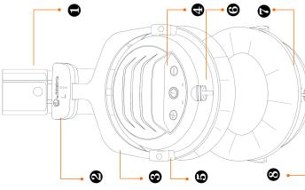
8 Wire audio input port 5 Tilting plastic part 6 Charging port 7 Ear cushion 1 Head band cushion 2 Slider plastic part 4 Control touch pad 3 Support folk
