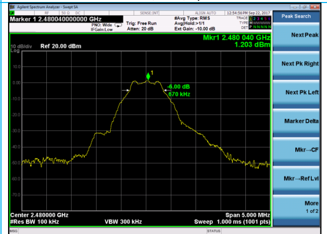
High Channel DTS BW, PSD, Spurious reference
