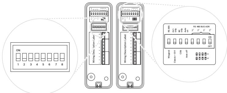
The reader has 8 DIP switches. Each switch is numbered from 1 to 8.
