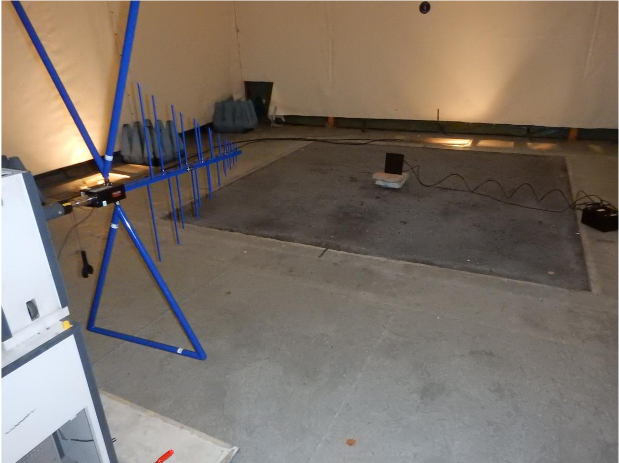
Figure 4, test setup photo for measuring lower frequency band of DUT. DUT is intentionally directed towards the measurement antenna.
