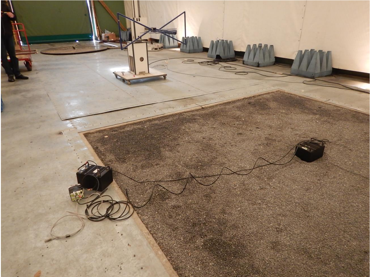
Figure 7, test setup photo showing measurements of horizontal polarized emission in the lower frequency band, photo taken from DUT-side of lab.
