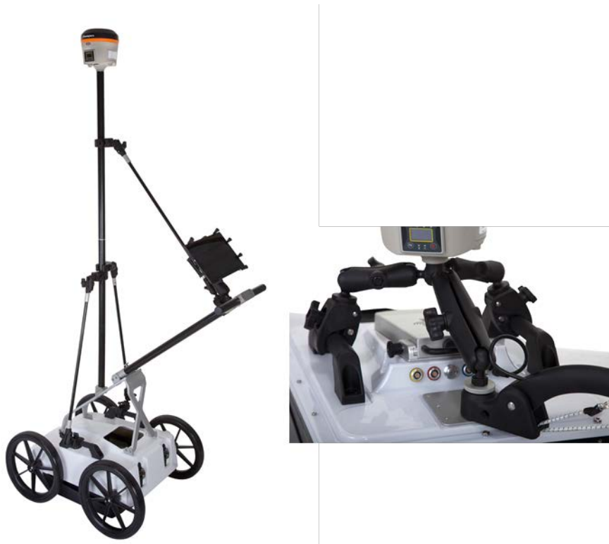
Figure 8 GPS-mounts for the Cart and antennas
