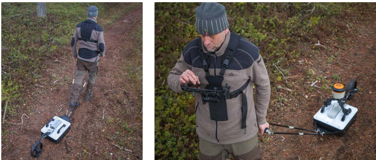
Figure 9 practical use of the waist belt, pulling rods, handle and pad-harness
