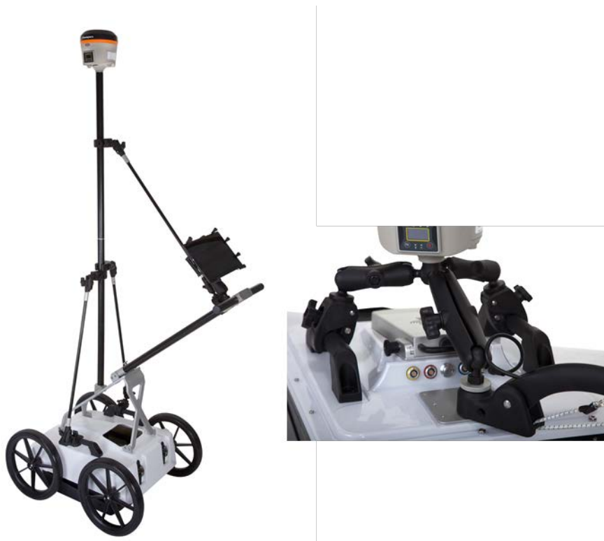
Figure 7 GPS-mounts for the Cart and antennas
