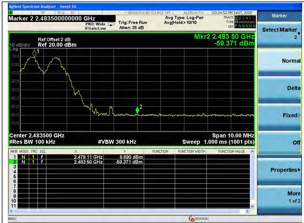
(Band edge with hopping on, Channel 78, GFSK)
