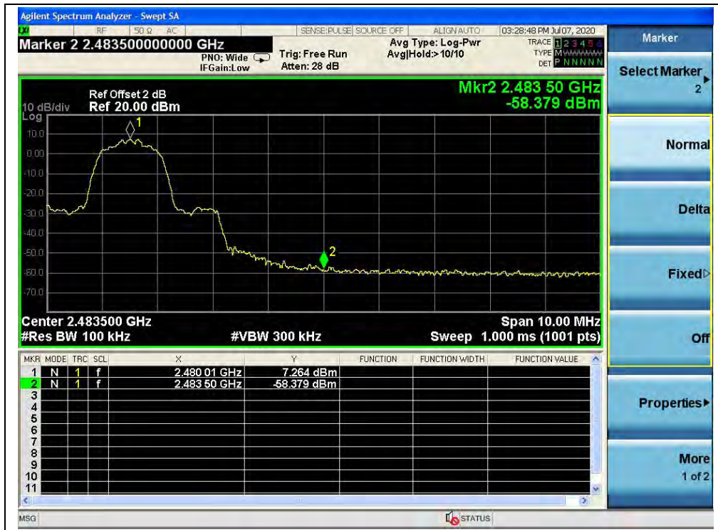
(Band edge, Channel 78, \pi/4 -DQPSK)
