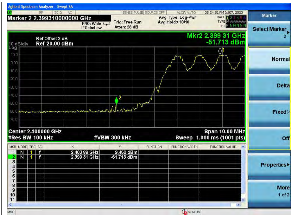
(Band edge with hopping on, Channel 0, GFSK)
