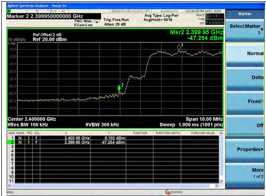
(Band edge with hopping on, Channel 0, 8-DPSK)
