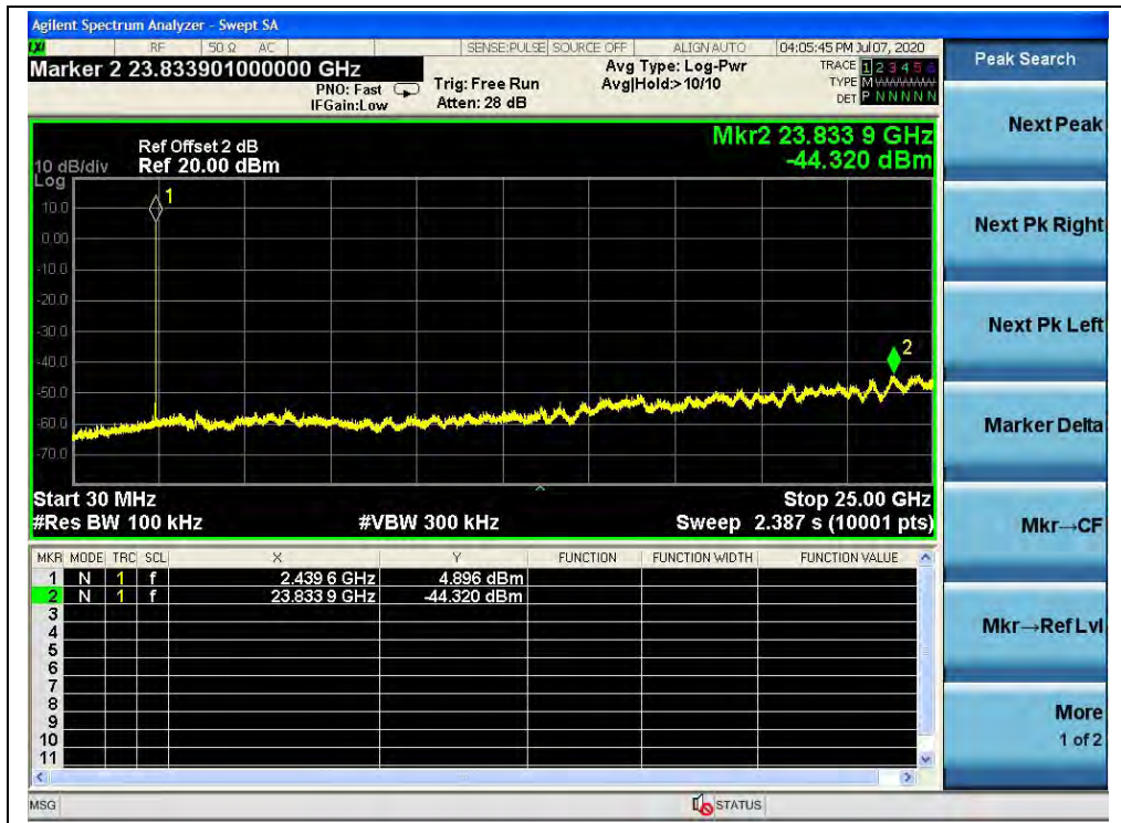
(30MHz to 25GHz, Channel 39, \pi/4 -DQPSK)
