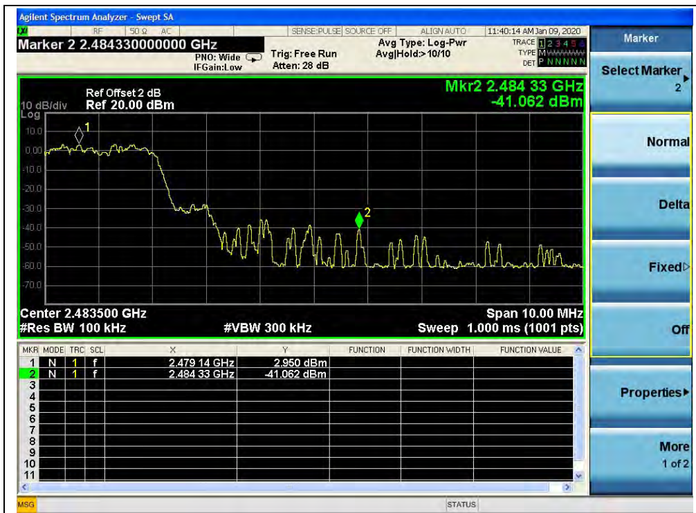
(Band edge with hopping on, Channel 78, 8-DPSK)
