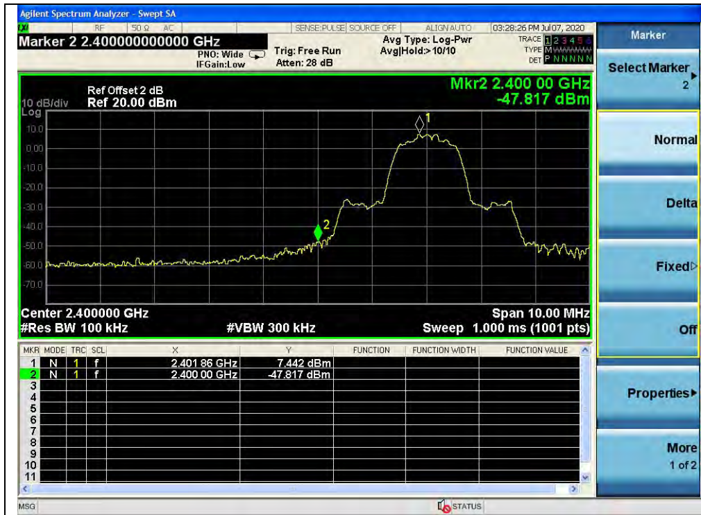
(Band edge, Channel 0, \pi/4 -DQPSK)
