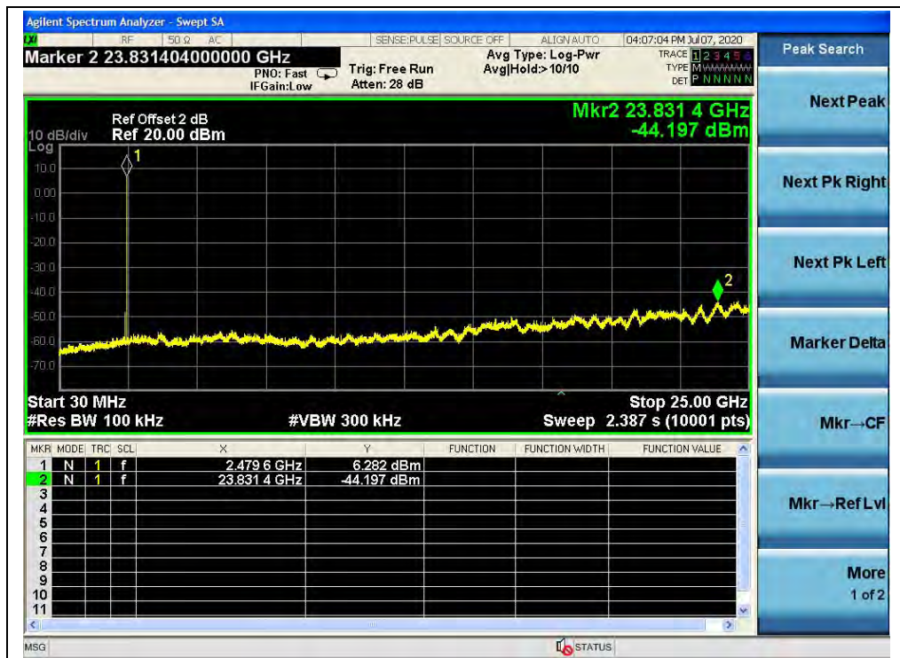
(30MHz to 25GHz, Channel 78, \pi/4 -DQPSK)
