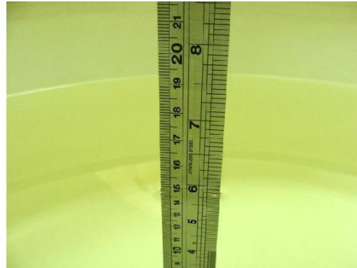
Fig 6.11 Photo of Liquid Height for Body SAR
