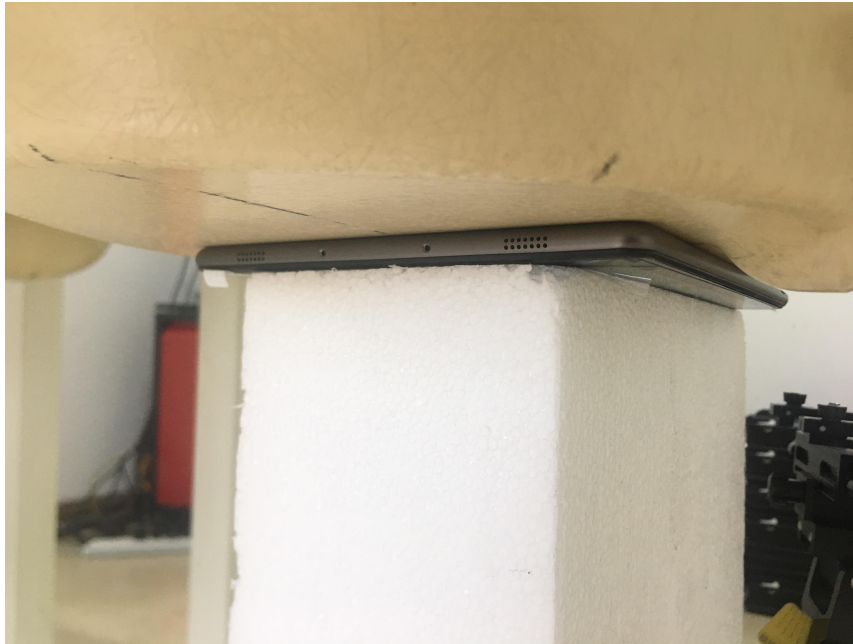
Back Side Without Holder (Test distance: 0mm, Thickness of DUT: 9mm)
