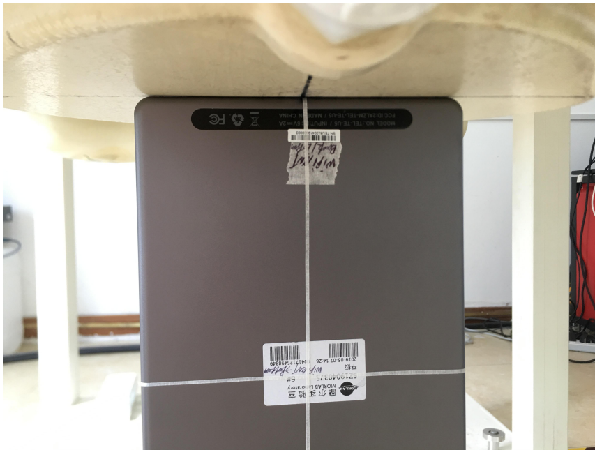
Bottom Side (Test distance: 0mm, Thickness of DUT: 9mm)
