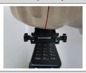
Photo 7: Back side 10mm with cover closed
