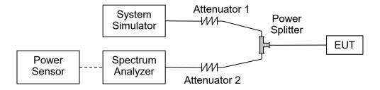
The EUTis coupled to the Spectrum Analyzer (SA) and the System Simulator (SS) with Attenuators through the Power Splitter; the RF load attached to the EUT antenna terminal is 500hm; the path loss as the factor is calibrated to correct the reading. The EUT is commanded by the SS to operate at the maximum output power. A call is established between the EUT and the SS.
