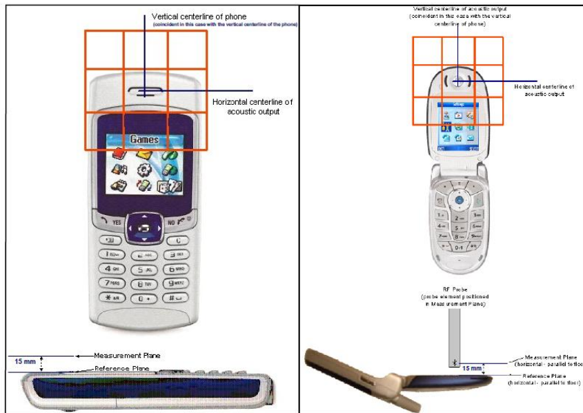
Fig 6.2 WD reference and plane for RF emission measurements
