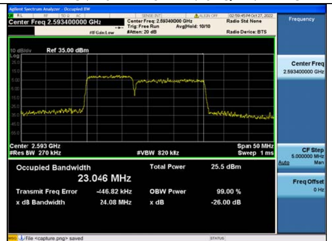
Band41C / 10MHz+15MHz / 16QAM/ Mid CH
